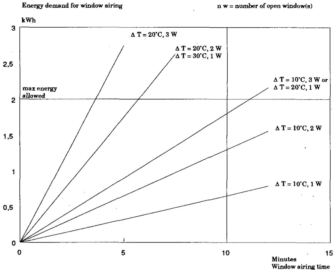
*Figure 8.12. Energy demand for window airing as a function of airing time in minutes for various temperature differences and number of opened windows. Airing demand is shown in table 8.4. The breadth of one window is 1.0 m*
