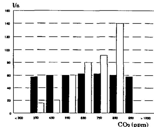
Flow rate as a function of CO<sub>2</sub> concentration. Average after DCV 49 l/s. Average before DCV 62 l/s.
