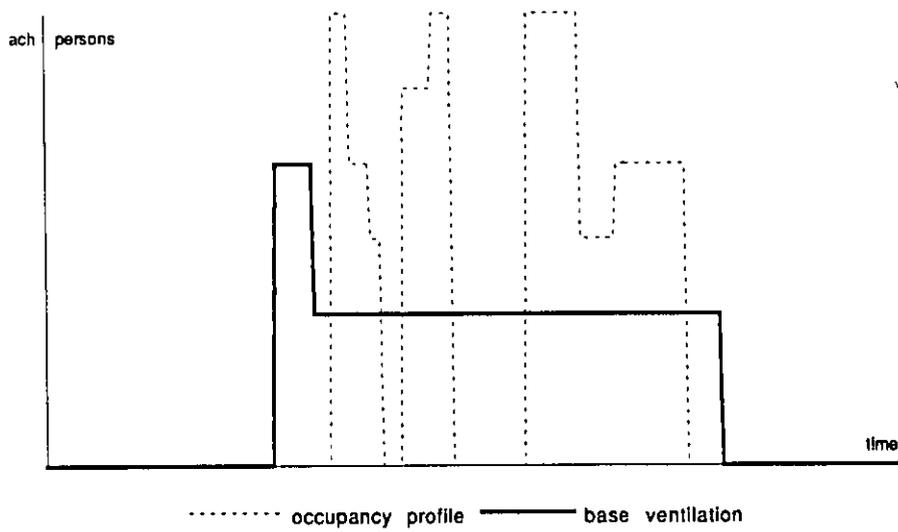
Figure 5.4. Pre-ventilation with higher ventilation rate
