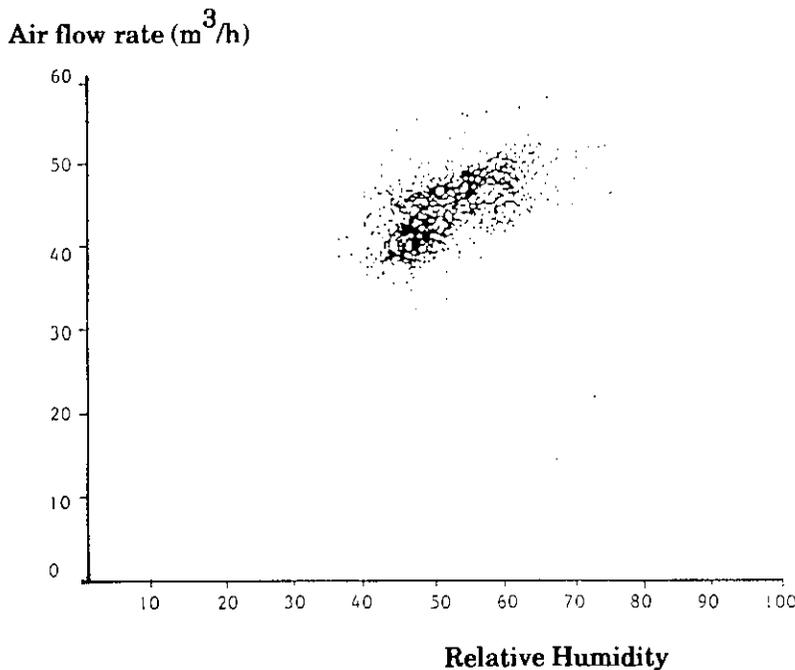
Figure 7.5. The air flow rate for a system governed by a RH-sensor, demonstration project Orsay, France.
