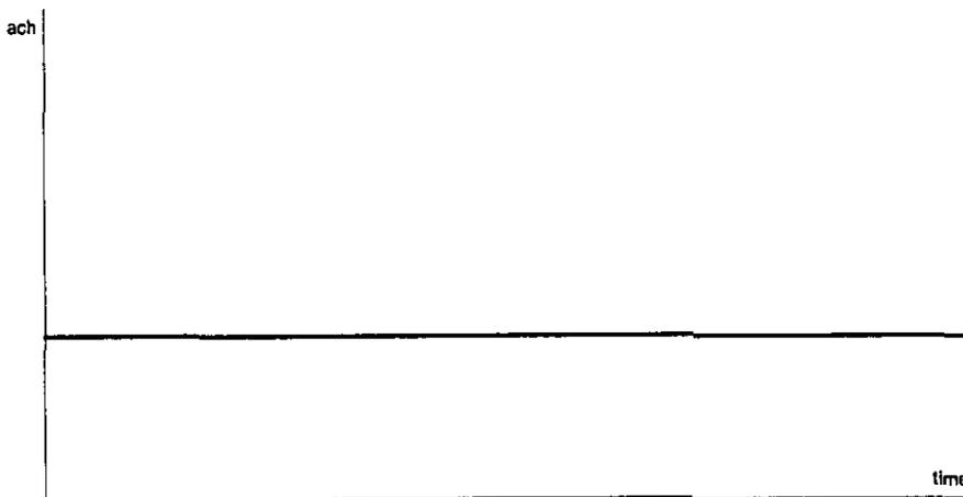
Figure 5.2. Constant 24-hour base ventilation
