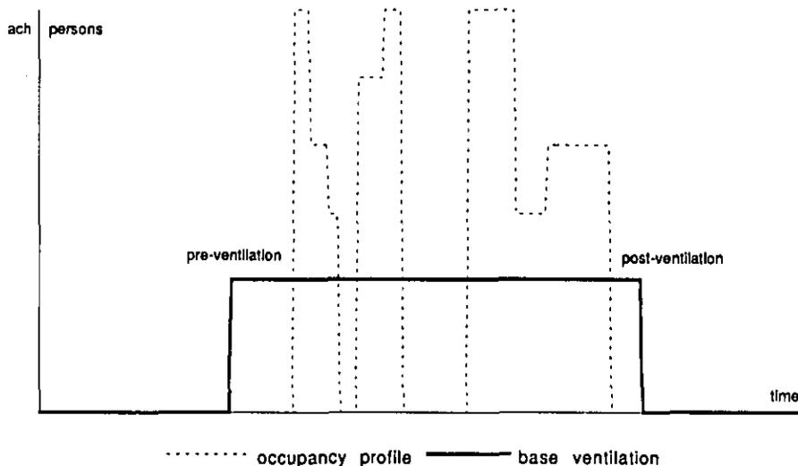
*Figure 5.3. Constant base ventilation rate during part-time with pre- and post-ventilation periods*
