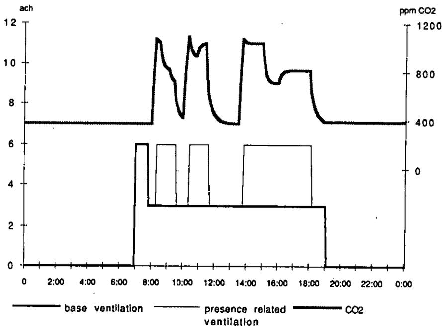
Figure 5.10. Ventilation operation with two-speed fan
