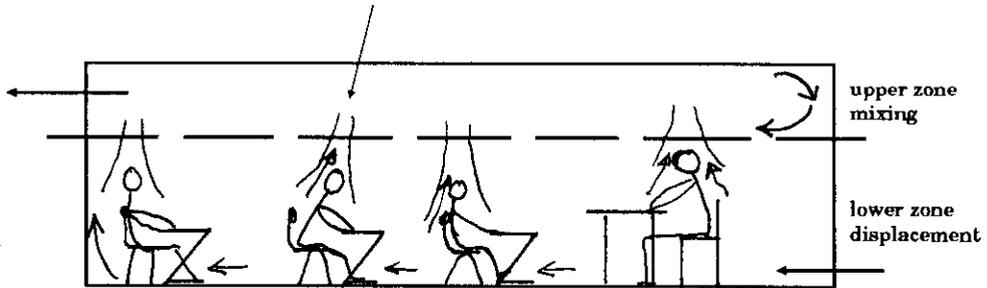
*Figure 8.6. Principle function of a ventilating system with displacement devices*
