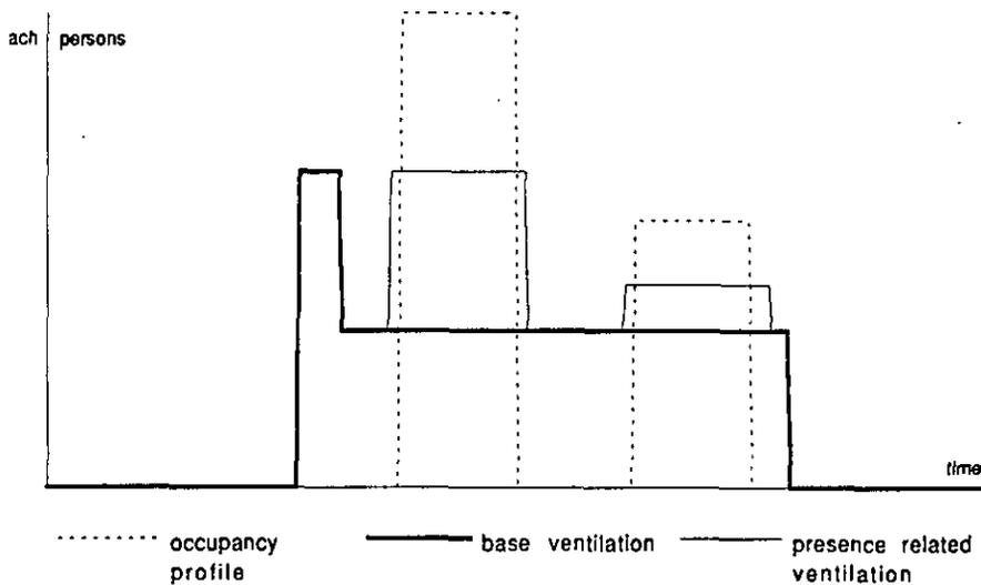
*Figure 5.7. Predictable occupancy with clock-controlled ventilation rate*
