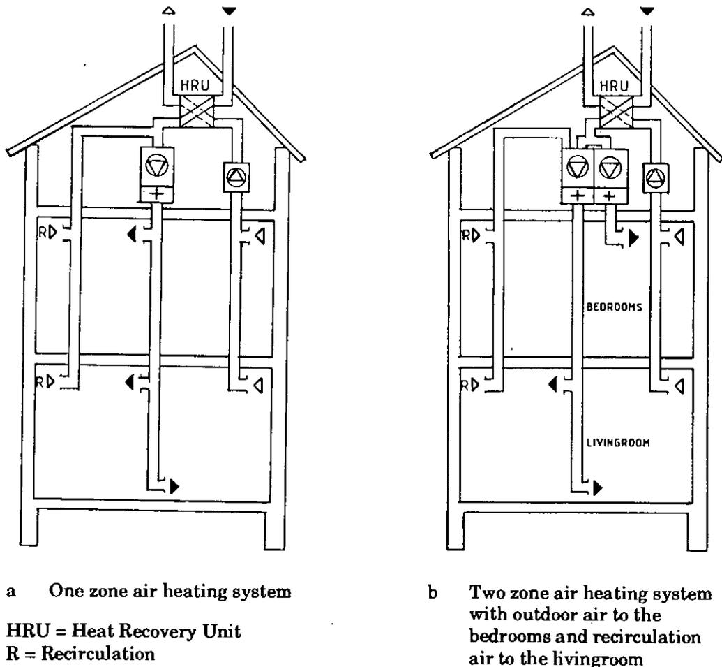
Figure 7.9. Mechanical ventilation combined with air heating.
