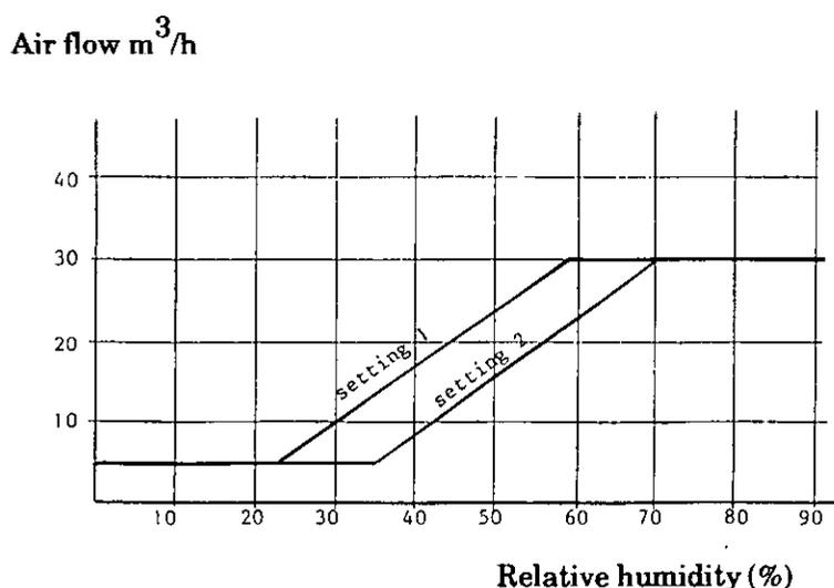
Figure 7.6 Flow rate through an air supply device furnished with humidity sensing control
