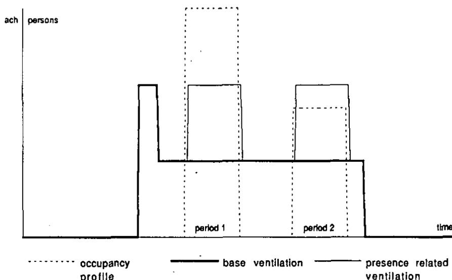
Figure 5.8. Adaptation of ventilation rate according to the presence
