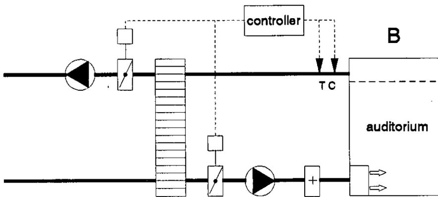
Figure 9.3. DCV system with throttling dampers.
