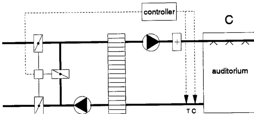
Figure 9.4. DCV system with return air
