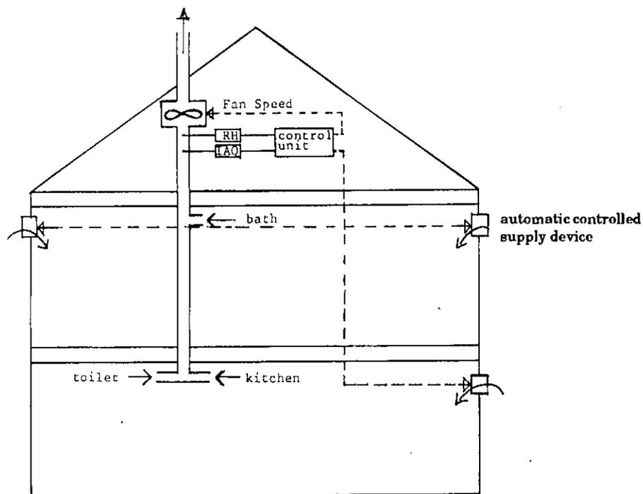
*Figure 7.7. A building furnished with a mechanical exhaust system. Fan speed and air supply devices are automatically controlled by relative humidity and /or air quality sensors.*
