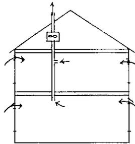
b Natural supply system and mechanical exhaust
