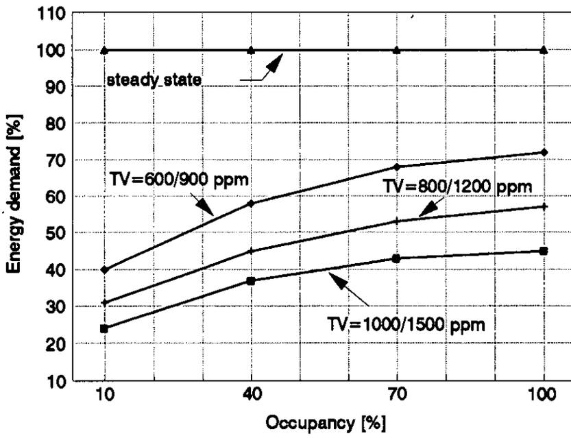
Figure 9.8. Energy savings in the auditorium HG D. TV=Threshold value
