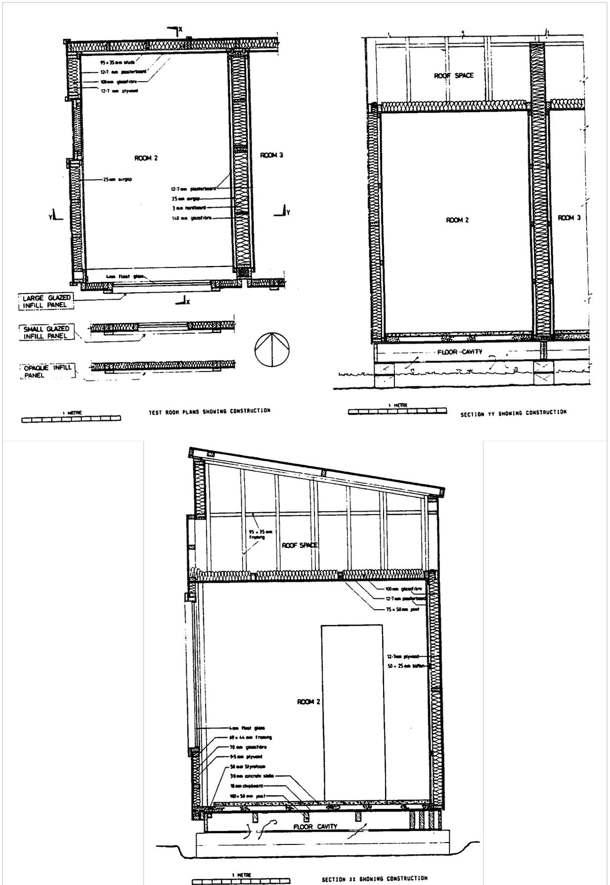
Fig. 11. Construction Details of the EMC Test Rooms
