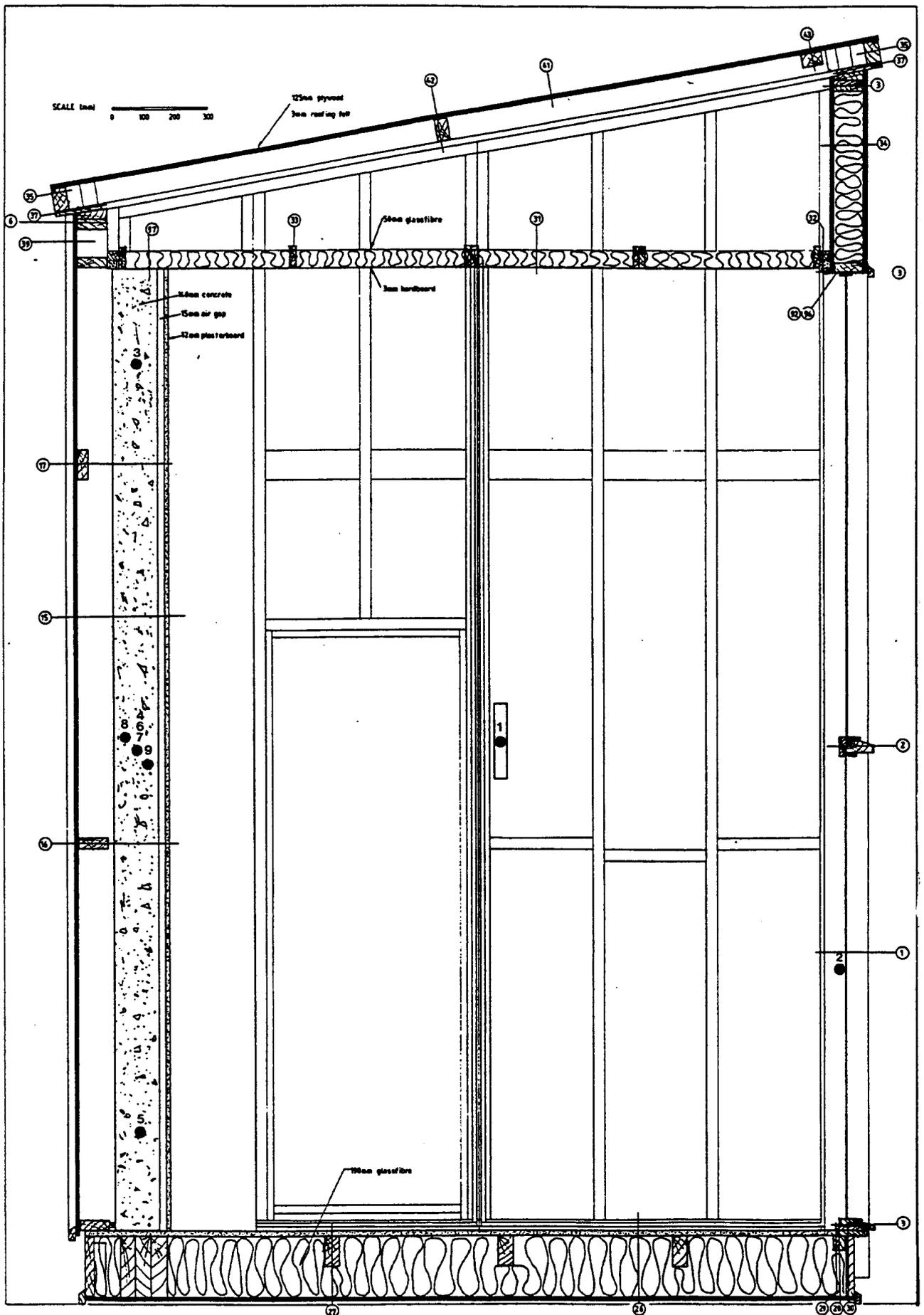
Fig.2. Vertical cross-section through Cell 1 looking east
