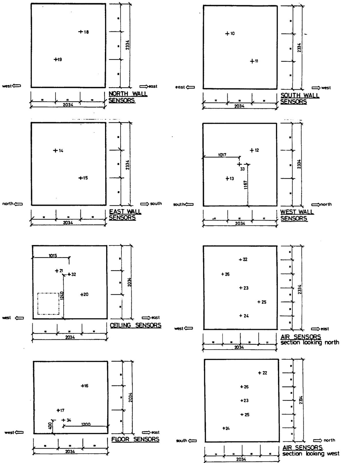
Fig. 5. Sensor locations in the British Gas test cell during the winter of 1985-86
