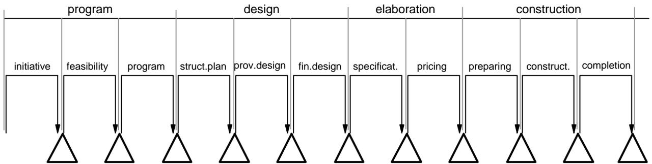
Figure 4: The design process subdivided into four stages and eleven phases<sup>1</sup>
