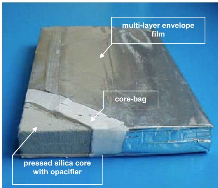
Figure 6: Components of a VIP. The core-bag provides mechanical stability for handling and protects the welding area from being polluted by core-powder.
