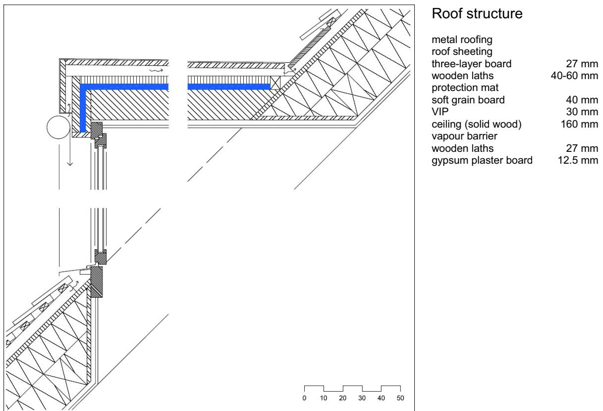
Figure 80: Vertical section through a prefabricated dormer window for the renovation of an old building
