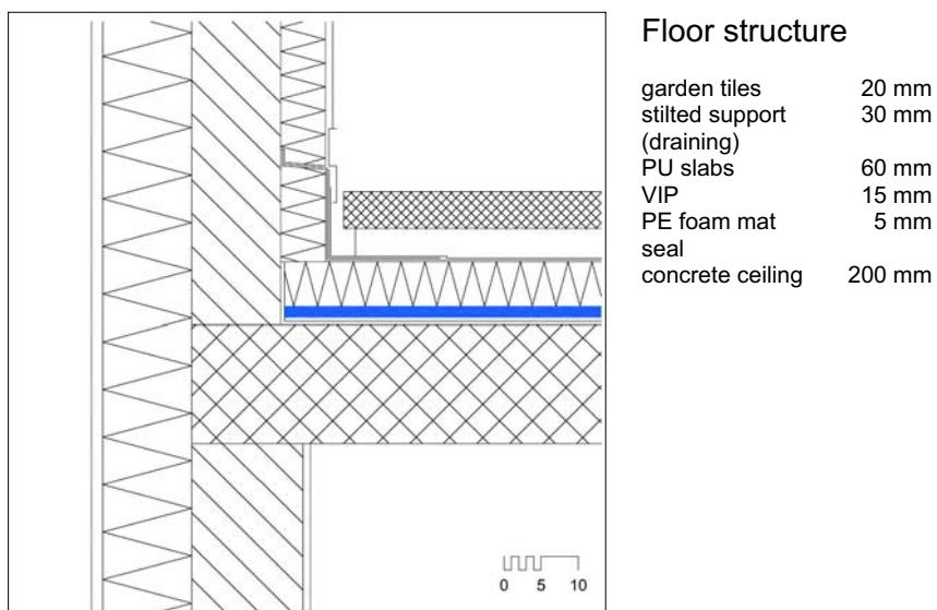
Figure 28: Vertical section through the joint detail at parapet
