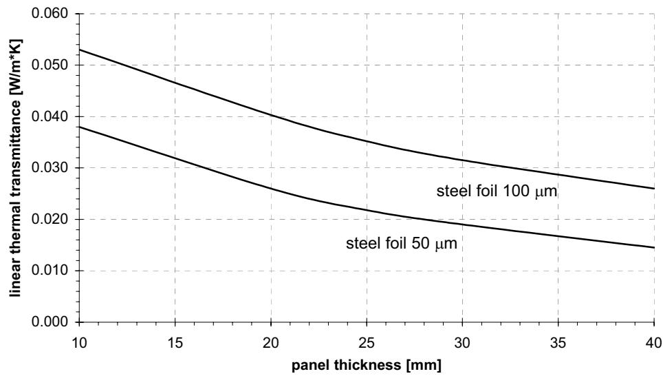
Figure 9: The effects of panel thickness and foil thickness on the linear thermal transmittance due to thermal bridging for a stainless steel foil ( $\lambda_{\text{foi}} = 25 \text{ W/(m}\cdot\text{K)}$ ;  $\lambda_{\text{cop}} = 4 \cdot 10^{-3} \text{ W/(m}\cdot\text{K)}$ ), based on numerical calculation
