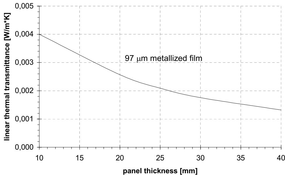
Figure 10: The effects of panel thickness on the linear thermal transmittance due to thermal bridging for a three layer metallized film;  $\lambda_{\text{cop}} = 4 \cdot 10^{-3} \text{ W/(m}\cdot\text{K)}$ ), based on numerical calculation
