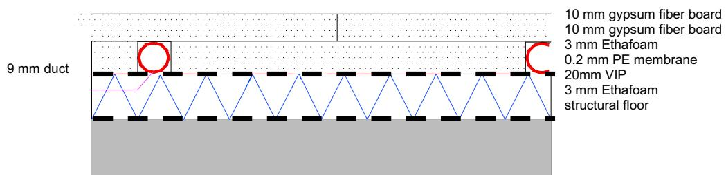
Figure 87: Principle construction layout of dry VIP based floor heating system (concept 2)
