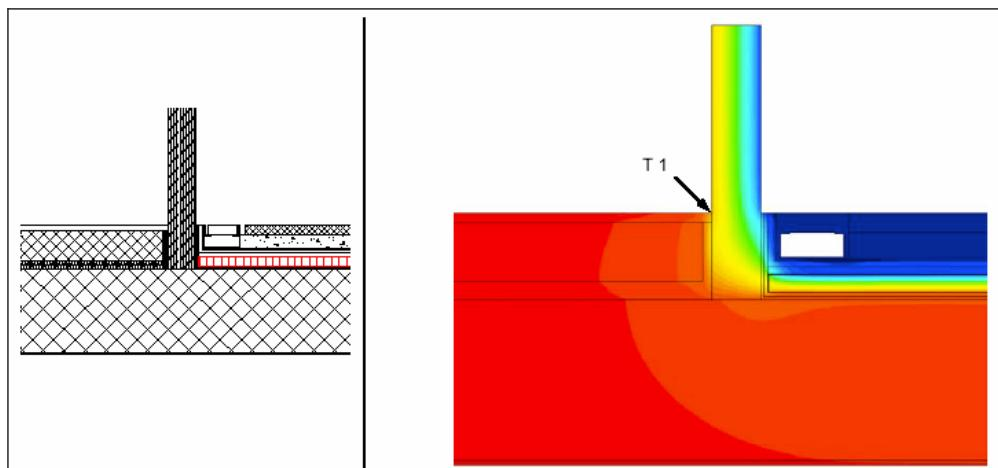
Figure 74: Vertical section through the terrace construction and threedimensional computational heatflow analysis. The calculated temperature  $T_1$  is  $14^{\circ}\text{C}$ .
