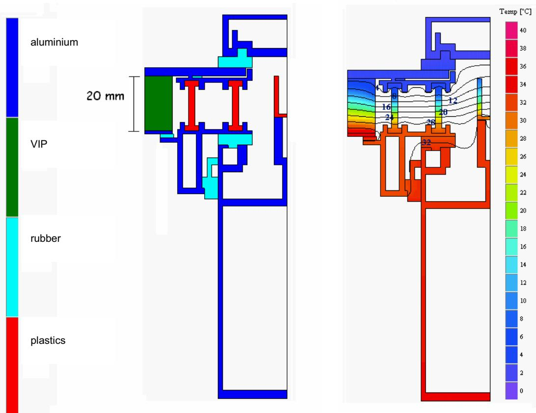
Figure 59: Left: Cross-section of the façade element without the radiator. The jamb-crossbar construction can be seen on the right hand side. The VIP is cut off on the left side.
