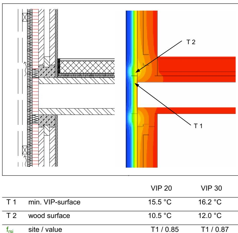
Figure 79: Vertical section through a joint of elements, three-dimensional computational heatflow analysis and calculated temperatures
