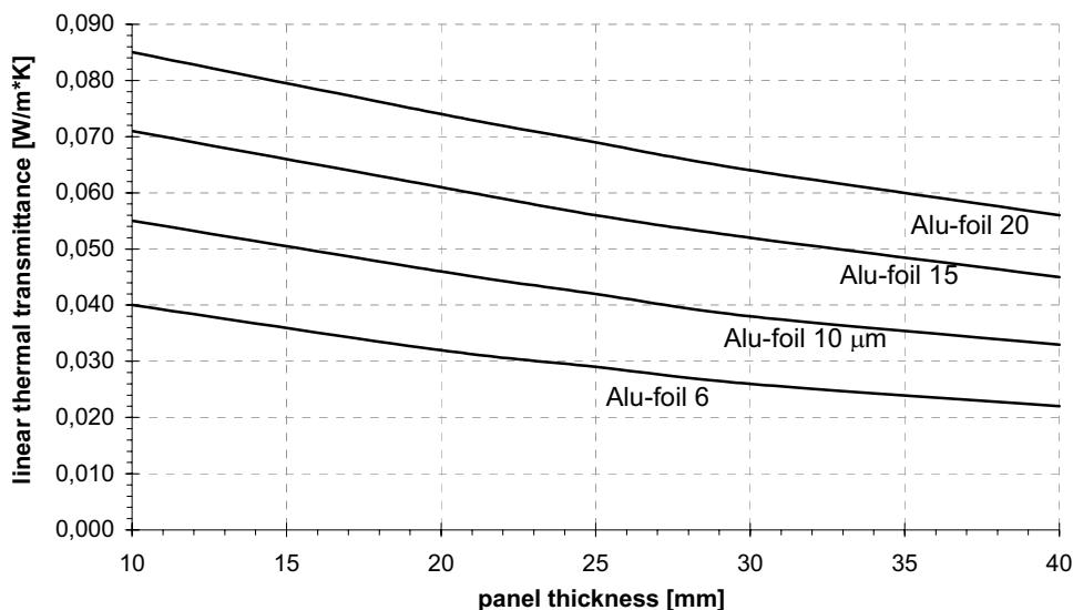
Figure 8: The effects of panel thickness and foil thickness on the linear thermal transmittance due to thermal bridging for an aluminium foil ( $\lambda_{\text{foil}} = 200 \text{ W}/(\text{m}\cdot\text{K})$ ;  $\lambda_{\text{cop}} = 4 \cdot 10^{-3} \text{ W}/(\text{m}\cdot\text{K})$ ), based on numerical calculation
