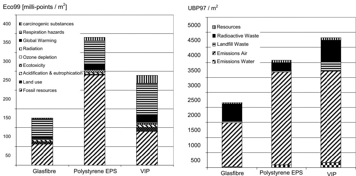
Figure 18: Left: Comparison of the categories of effects for the insulating materials glass wool, polystyrene EPS and VIP according to the method Eco-indicator 99
