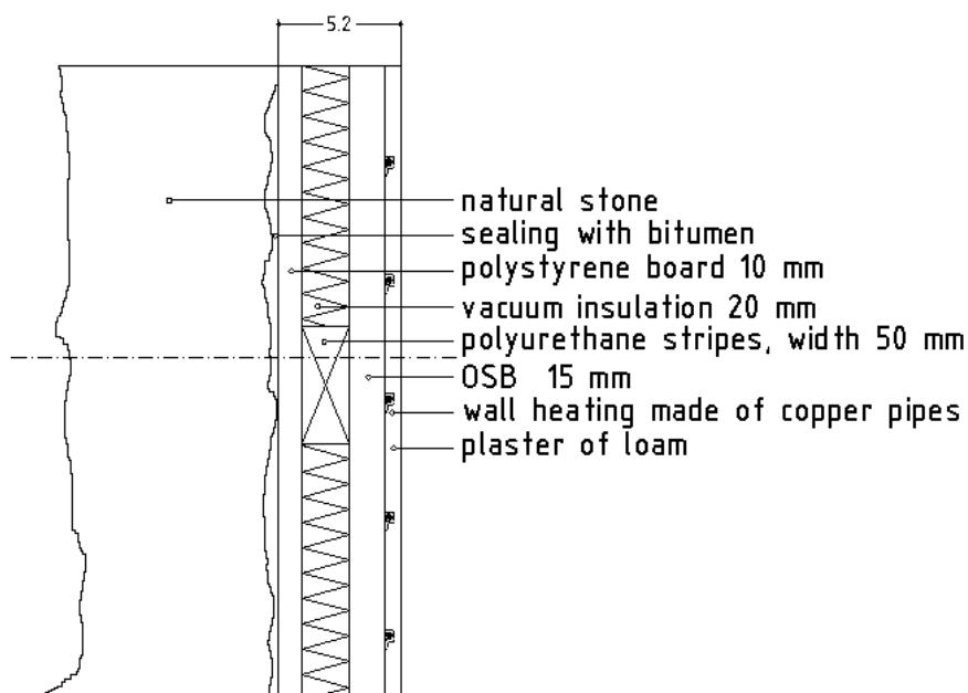
Figure 51: Cross-section of the wall
