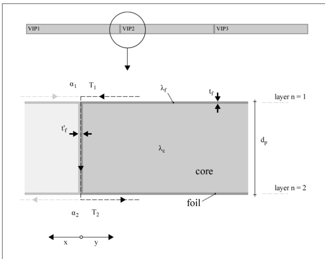
Figure 12: Schematic representation of the thermal bridge due to an aluminium high barrier foil
