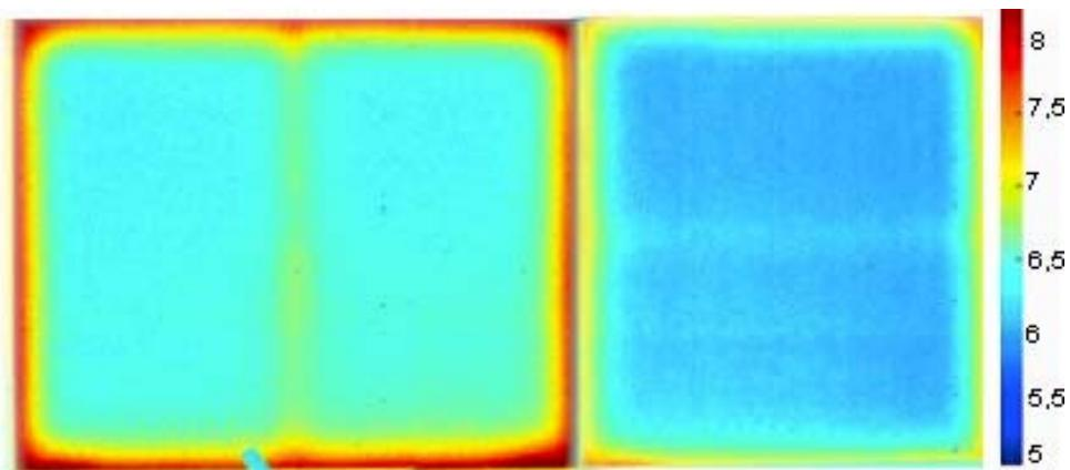
Figure 55: Infra-red image of two elements. On the left hand side the spacer is made of stainless steel and on the right hand side the spacer is made of Purenit.
