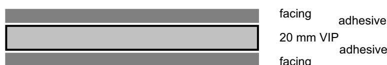
Figure 17: The layout of sandwich panels
