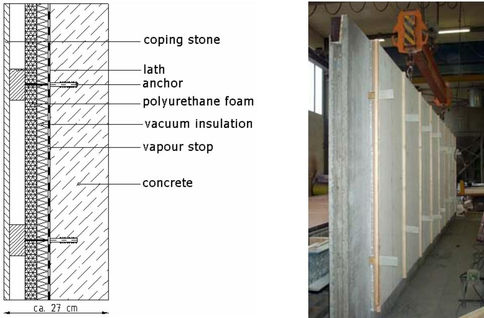
Figure 61: Left: Intended design for the prefabricated wall elements. An average U-value of 0.15 W/(m<sup>2</sup>·K) is achieved with a total thickness of only 27 cm.
