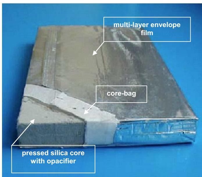
Figure 1: Components of a VIP. The core-bag provides mechanical stability for handling and protects the welding area from being polluted by core-powder
