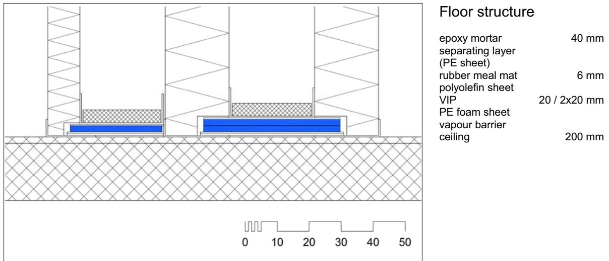
Figure 31: Vertical section of a cold (left) an a deep-freeze room (right)
