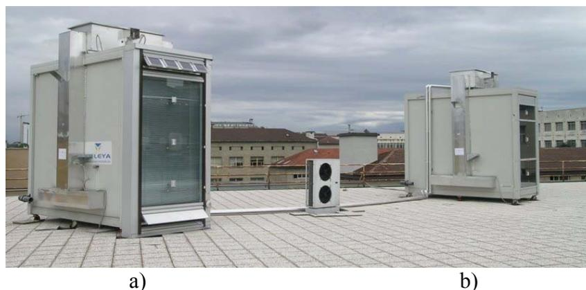
**Figure 4.16 – pictures of: a) Façade under test (in this case a hybrid ventilated façade), b) Reference façade.**
