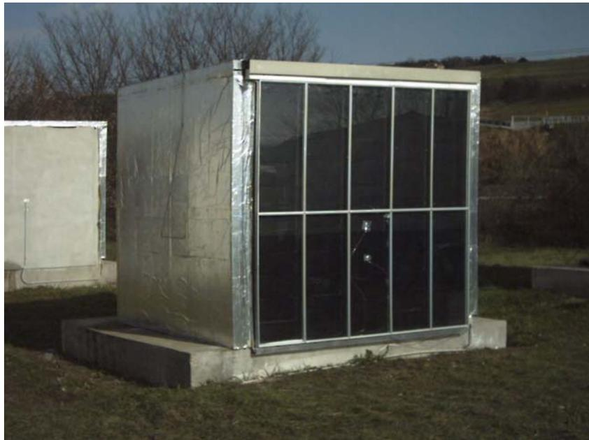
***Figure 7.6 – Example of an experimental passive solar wall making use of PCM (Experimental test facility at Università Politecnica delle Marche - Italy).***
