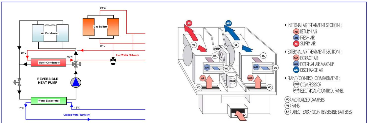
*Retrofit options 1 (left – dual condenser heat pump) and 2 (right – air-to-air heat pumps)*
