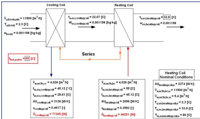
*AHU coils series change over: the cooling coil is used as a secondary heating coil and allows reaching the temperature setpoint with low temperature hot water (50°C) by increasing the heat transfer area.*
