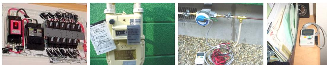
*Figure 2-108: Measuring instruments (a, b, c and d from left to right: electricity, gas, kerosene and air temperature)*
