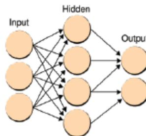
Figure 2-58: Feed-forward neural network topology
