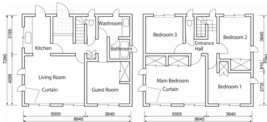
Figure 4-1: Typical residential building geometry used in Japan (Udagawa, 1985)
