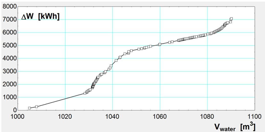
Figure 7-34: Electricity consumption as function of the water consumption
