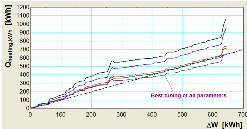
Figure 7-20: Simulated heating demand as function of the electricity consumption
