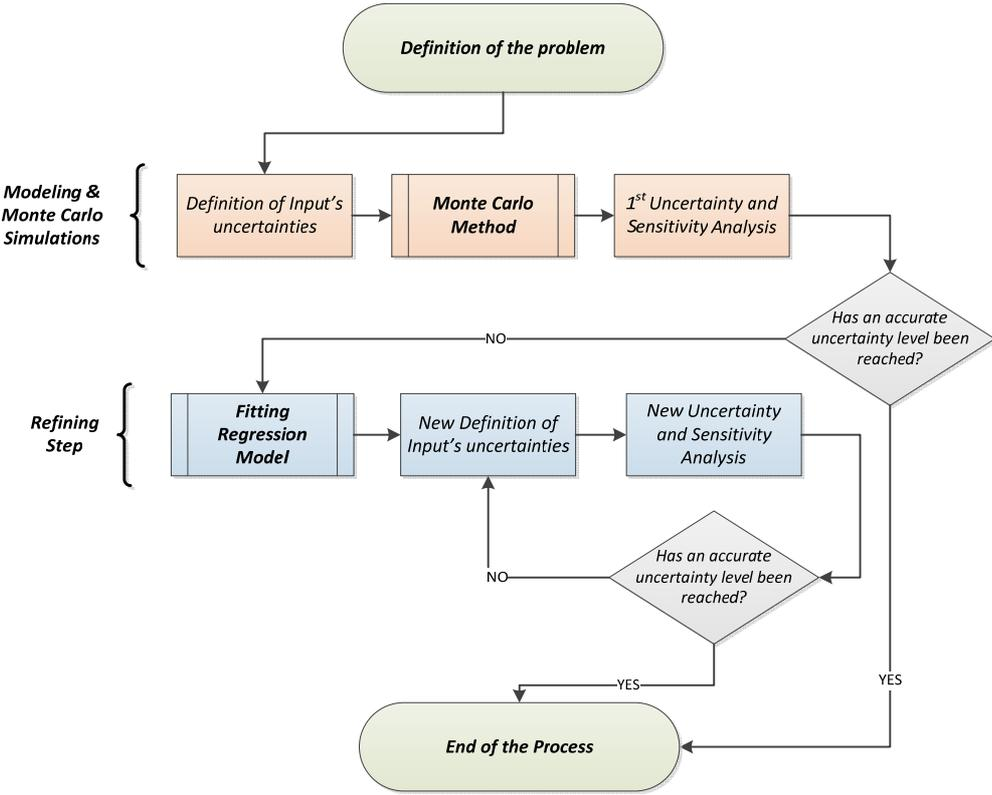
Figure 7-2: Proposed methodology combining sensitivity analysis and disaggregation of output variance
