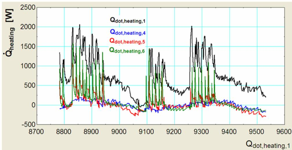
Figure 7-30: Simulated heating demands after best tuning of all parameters
