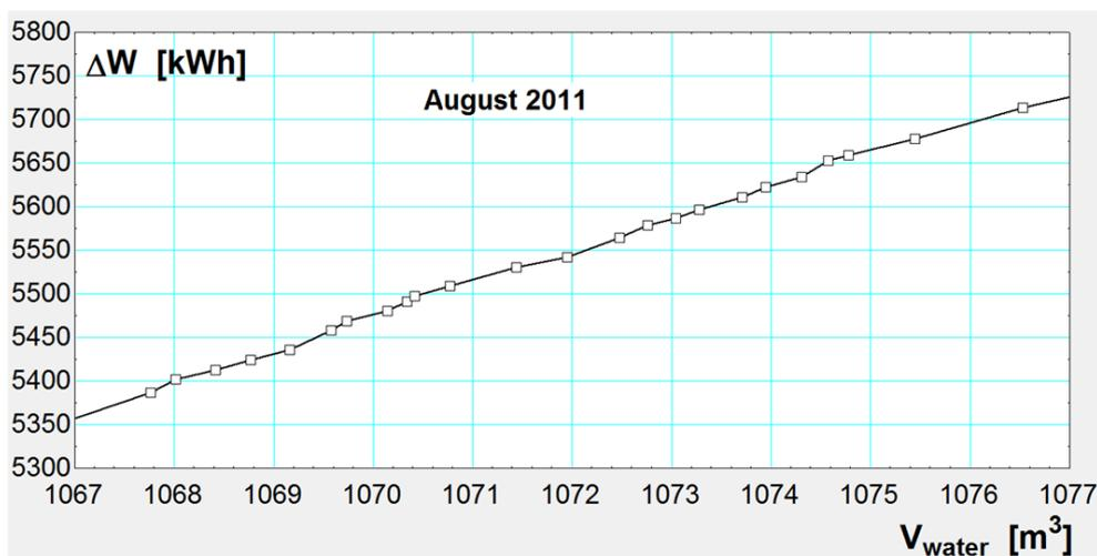
Figure 7-35: Electricity consumption as function of the water consumption in August 2011
