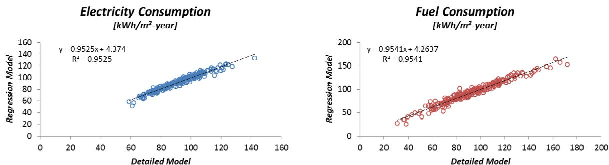
Figure 7-11: Detailed model versus regression model predictions.
