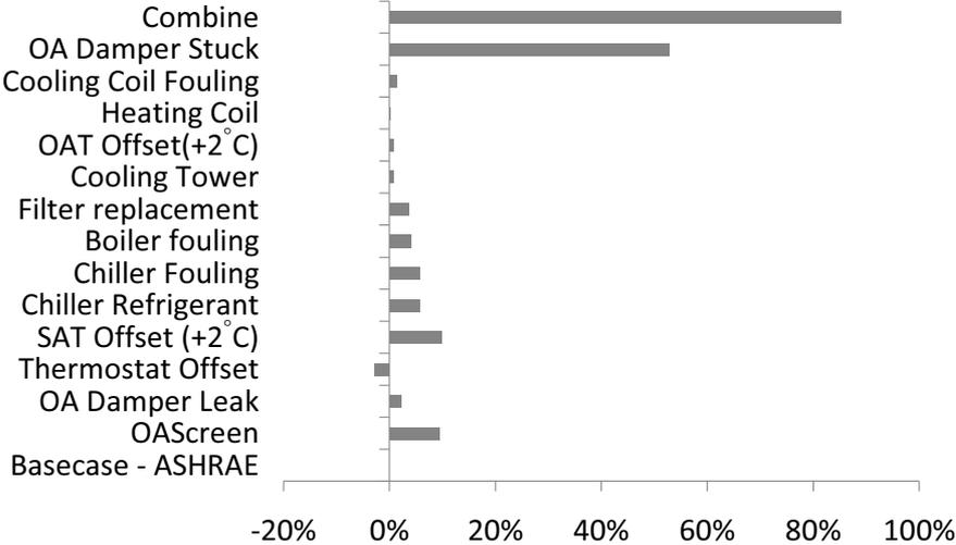
Figure 7-37: The impacts of poor HVAC maintenance on HVAC source energy consumption for a large office building in Chicago, USA
