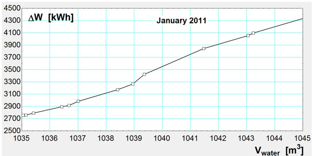
Figure 7-36: Electricity consumption as function of the water consumption in January 2011
