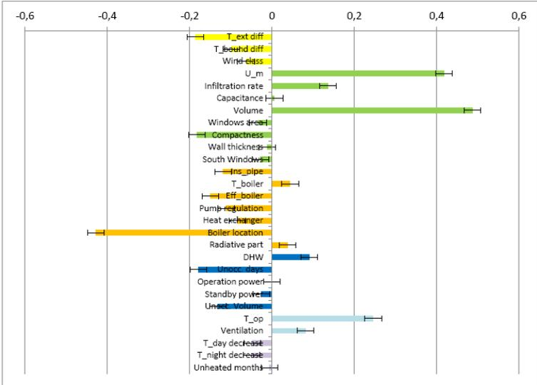
Figure 5-1: Example of results obtained with the Morris statistical method and showing sensitivity of different parameters
