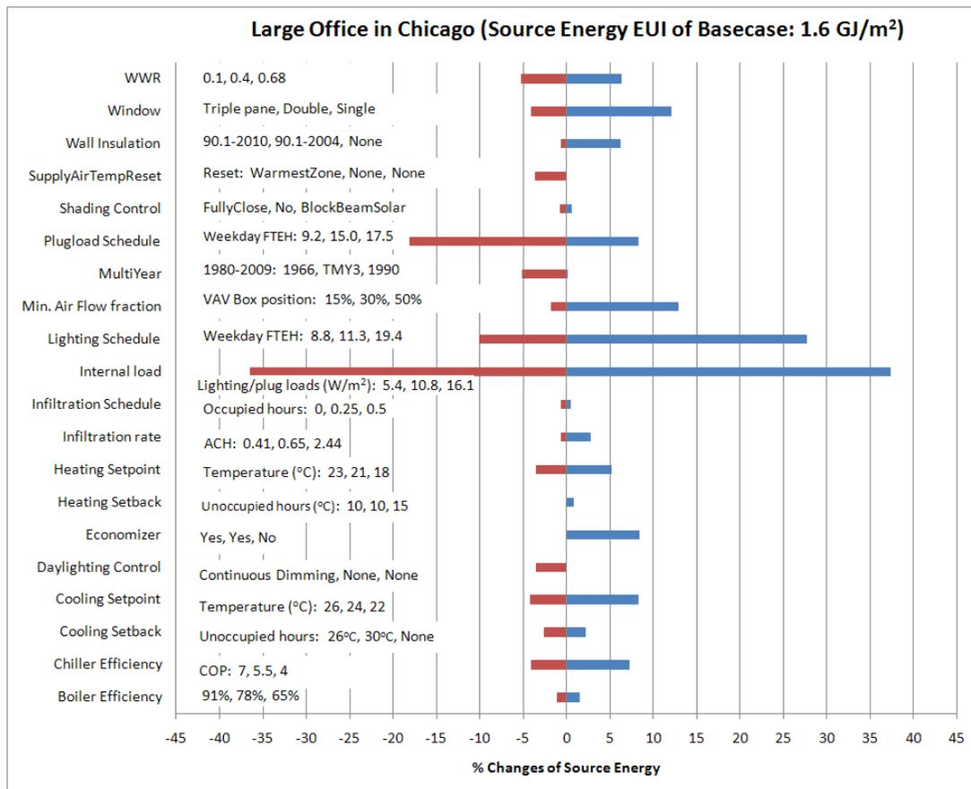
Figure 5-3: Example of sensitivity analysis applied to an office building in the US
