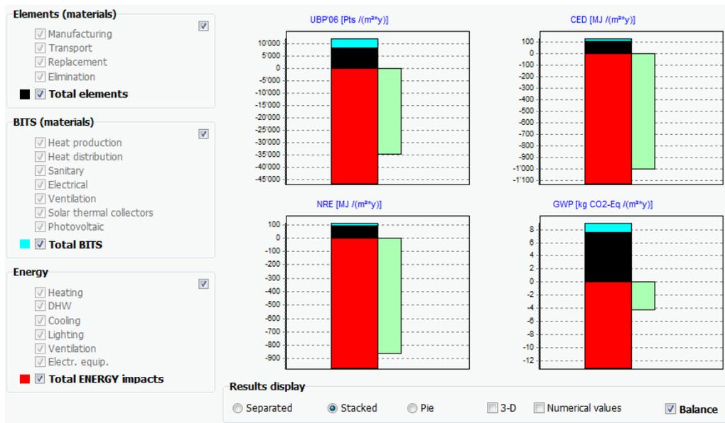
Figure 12 Annex 56 energy-related renovation LCA balance
