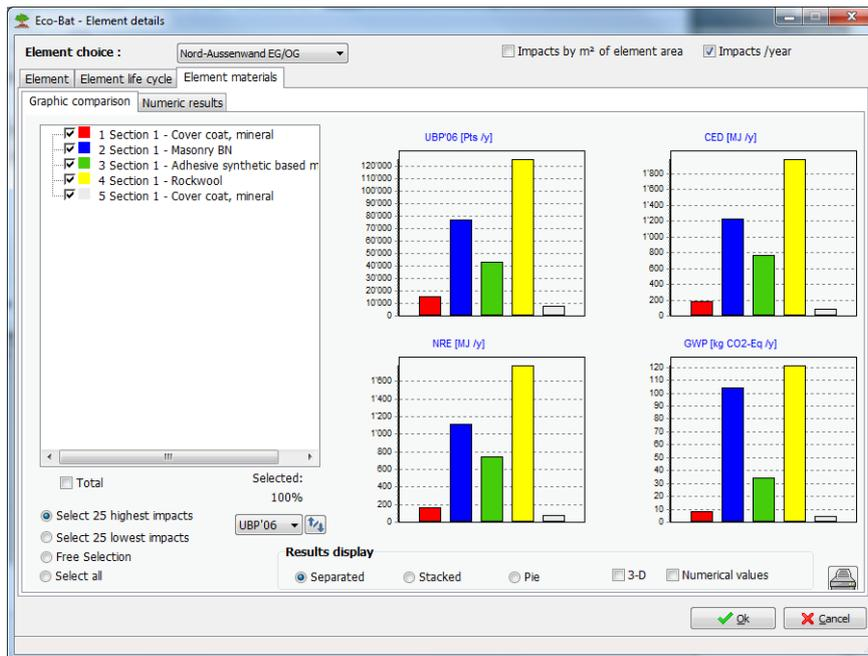
Figure 11 LCA comparison of a construction element's materials
