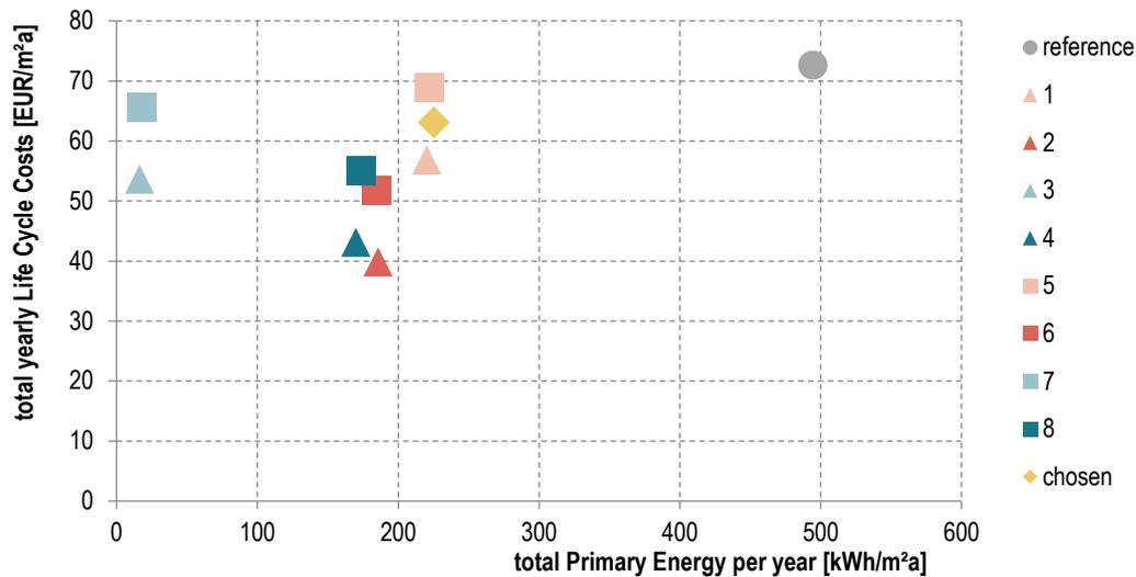
Figure 17 Results for the total primary energy for all the analysed renovation packages
