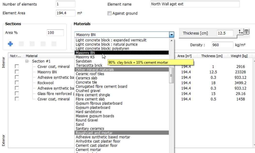
Figure 10 Definition of a construction element
