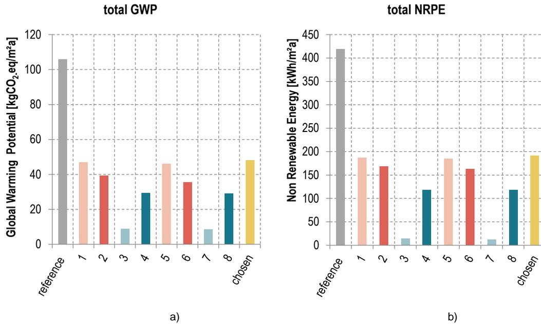
Figure 16 a) Graphic results of the GWP analysis and b) NRPE for the renovation measures
