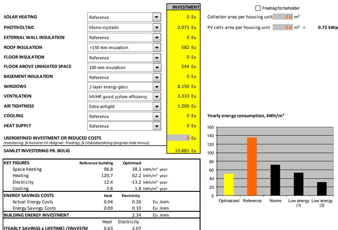
Figure 5 Example of ASCOT results for optimization of a building renovation with Annex56 methodology (Mørck, 2015)
