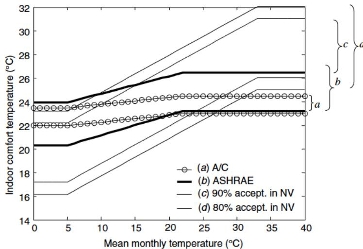
**Figure 2.2.** Comfort range for air conditioning and for natural ventilation: (a) air conditioning; (b) ASHRAE comfort range; (c) natural ventilation, 90% acceptability limits; (d) natural ventilation, 80% acceptability limits. [4].
