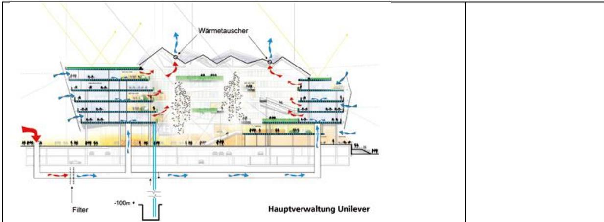
Figure 5.18. UNILEVER central administration building with exhaust atria, Hamburg, Germany
