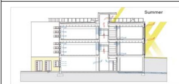
Cross and vertical ventilation systems acting together with the buried pipes system
