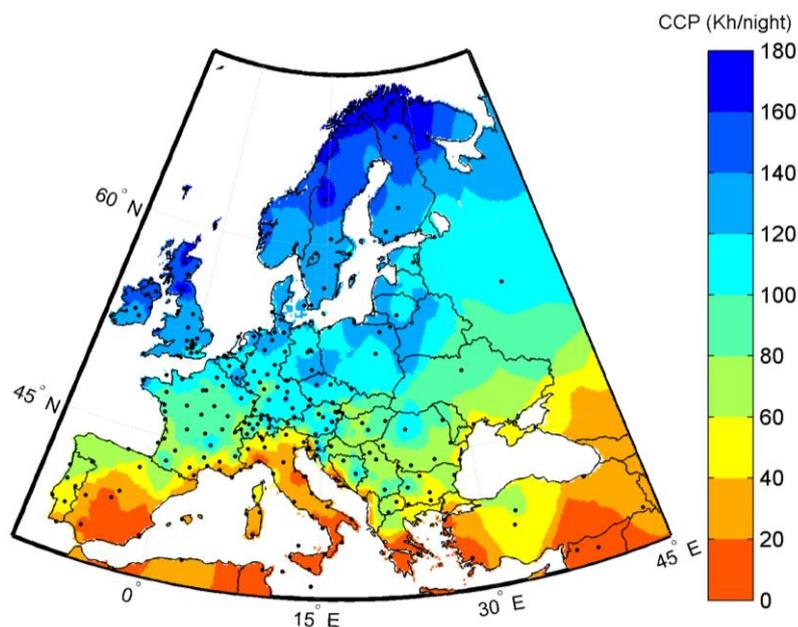
**Figure 2.5.** Map of mean climatic cooling potential (Kh/night) in July based on Meteonorm data [13].
