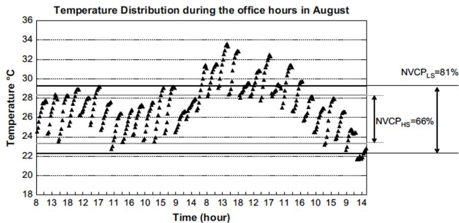
**Figure 2.11.** Temperature distribution and natural ventilative cooling potential of a Low-Energy Demonstration Building in Beijing in August, depending on the selected comfort criteria, [8].
