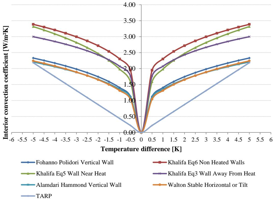
Figure 6-5. Vertical wall interior convection model comparison at different temperature differences between air and wall interior surface. Source: Belleri A. [49]
