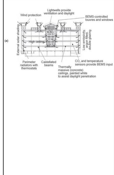
**Components used for ventilative cooling (see chapter 5 for examples)**
