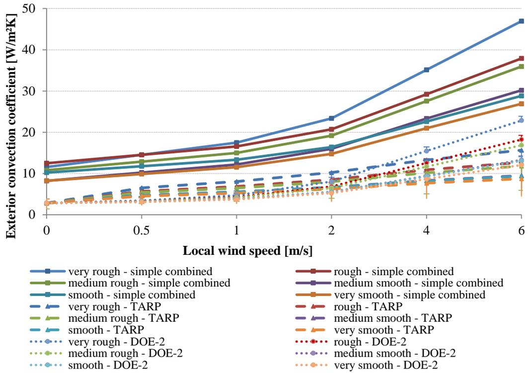
Figure 6-4. Vertical wall exterior convection model comparison depending on wind speed and surface roughness at a temperature difference of 10K between outdoor air and external wall surface when the façade is directed windward. Source: Belleri A. [49]
