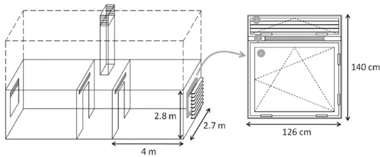
**Figure 2.14.** Overview of office geometry with shading device and design of the passive stack night ventilation openings with detail of the fenestration system (1: Operable window; 2: self-regulating ventilation grill; 3: night ventilation inlet opening), [32].
