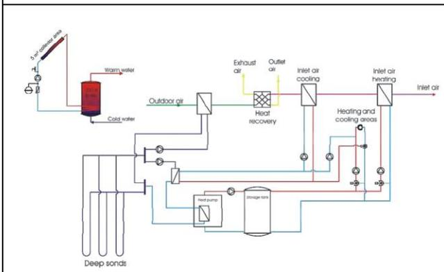
**Schematic arrangement of the heating/cooling system**
