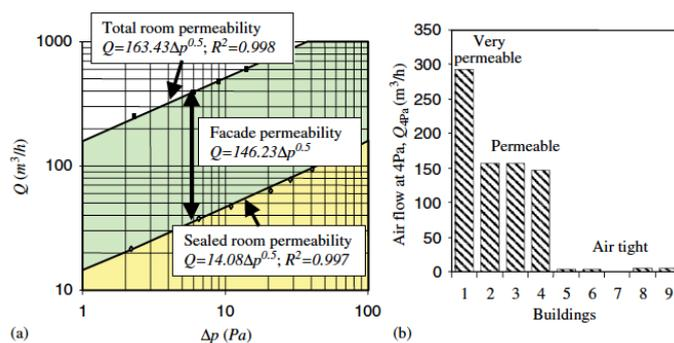
**Figure 2.13.** Building permeability for nine school buildings used in experiments on indoor/outdoor pollution ratio ([27], original data from [31]).
