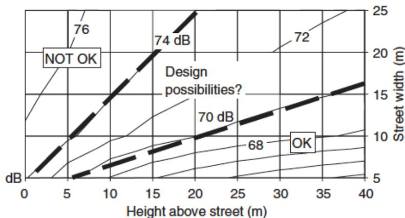
**Figure 2.12.** Contours of noise level at different heights above the street and street widths. Configurations in which natural ventilation is possible are indicated (OK), as are those in which it is ruled out (NOT OK). Between these two extremes is a region in which there are possibilities for design solutions. [30].
