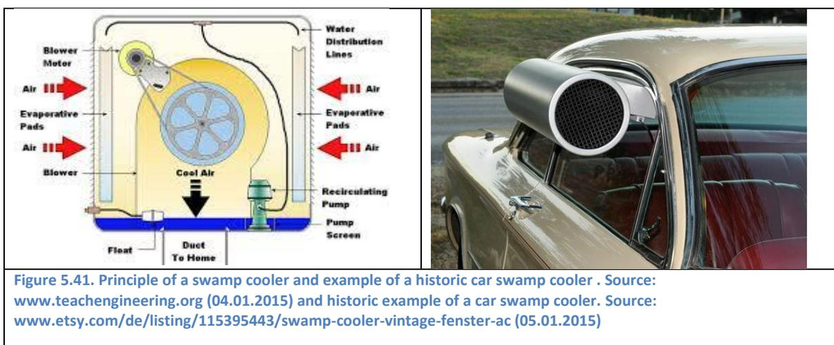
Figure 5.41. Principle of a swamp cooler and example of a historic car swamp cooler . Source: [www.teachengineering.org](http://www.teachengineering.org) (04.01.2015) and historic example of a car swamp cooler. Source: [www.etsy.com/de/listing/115395443/swamp-cooler-vintage-fenster-ac](http://www.etsy.com/de/listing/115395443/swamp-cooler-vintage-fenster-ac) (05.01.2015)
