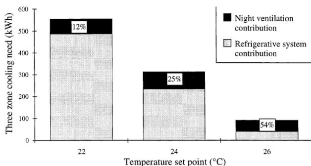
**Figure 2.15.** Daytime cooling needs of rooms A, B and C with and without night ventilation. [33].
