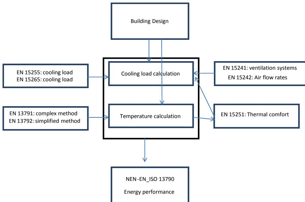
**Figure 3.1:** From Design to Energy performance Value in accordance with the European Union Standards.
