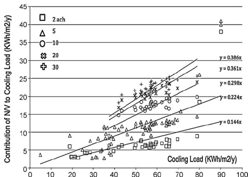
**Figure 2.19.** Calculated energy contribution of night-time ventilative cooling as a function of the initial cooling load for various levels of air flow rates, [37].
