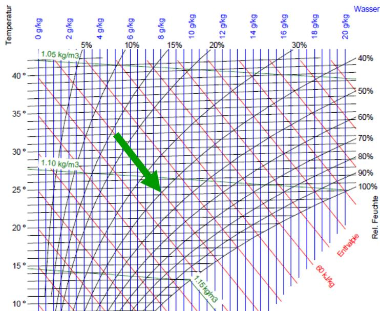
Figure 5.40. Process of evaporative cooling within the psychrometric chart
