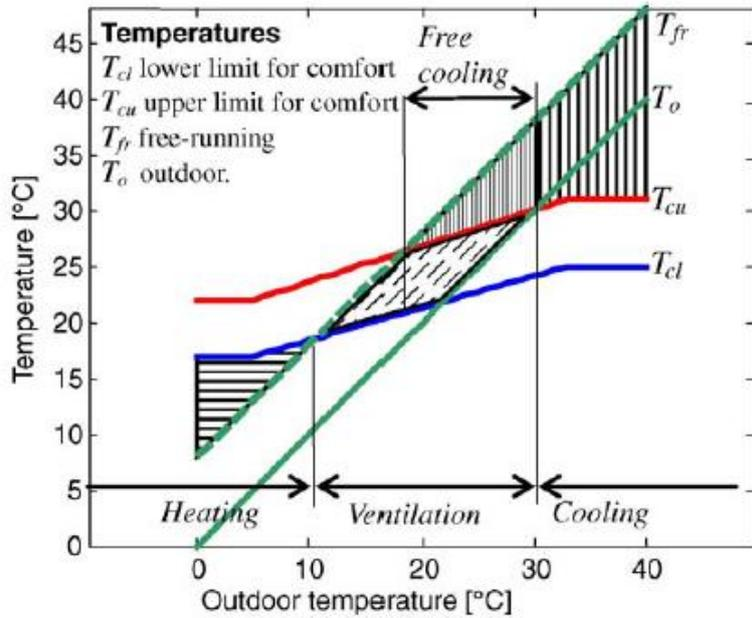
**Figure 2.1.** Ranges for heating, free-cooling and mechanical cooling when the free-running temperature is higher than the outdoor temperature. [4].
