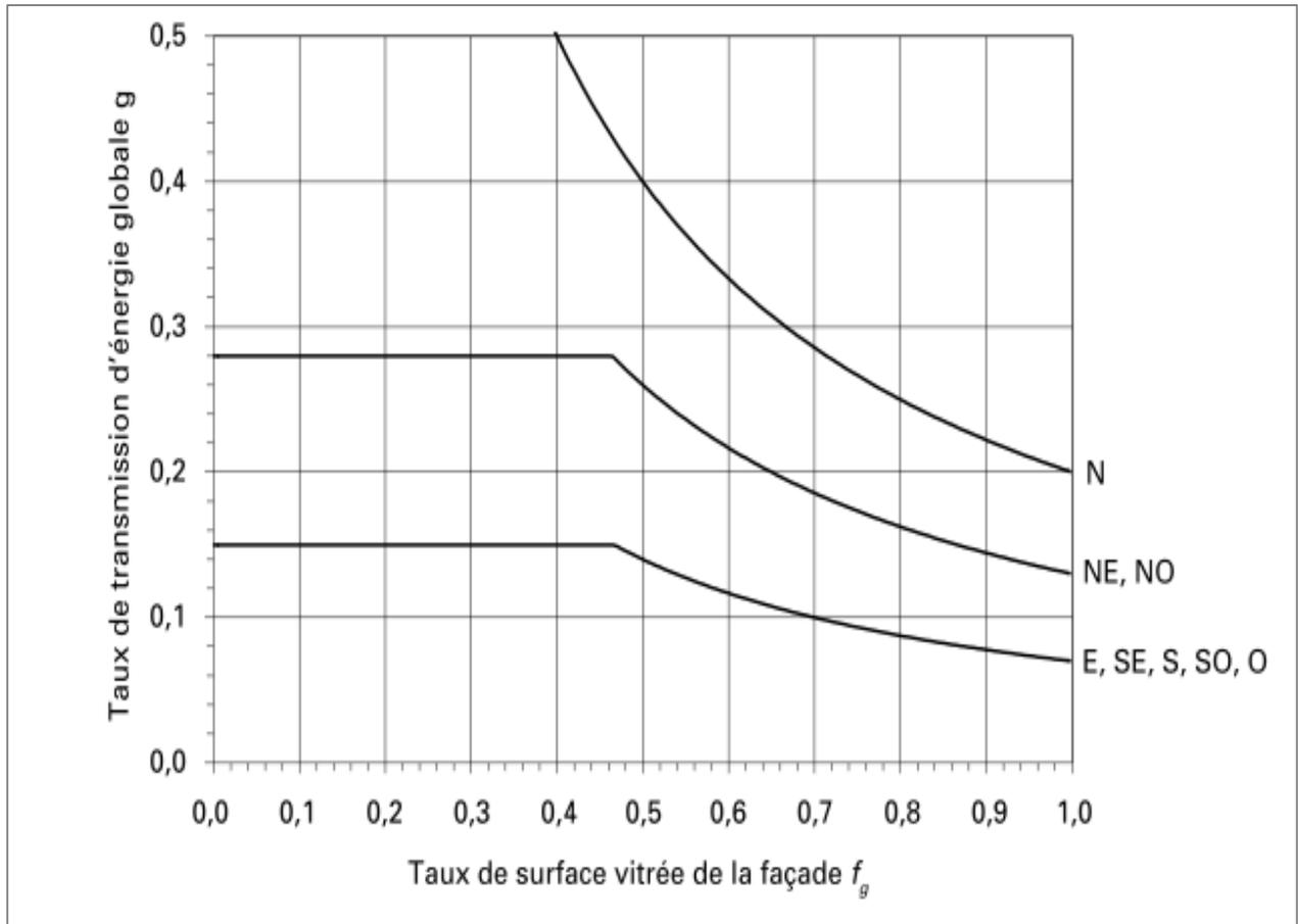
Figure A1: Requirements on solar shading in the Swiss regulations:
