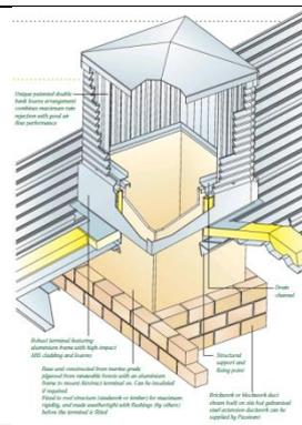
Figure 5.26. Powerless wind turbine ventilator. Airier Natura Pvt. Ltd., Bangalore, India. Source: <http://www.industrialairventilator.com/> (31.12.2014)
