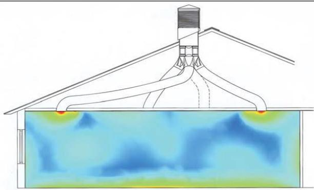
Figure 5.33. Modern bi-directional windcatcher with option for ducted air dispersal by Passivent, UK
