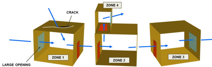
Figure 6-1. Airflow network schematic representation. Source: IBPSA-USA
