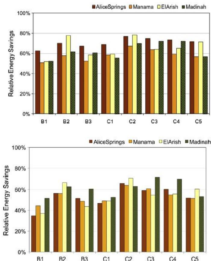
**Figure 2.17.** Savings in plant energy due to the application of hybrid cooling strategies for low (upper figure) and high (lower figure) internal heat gain relative to energy use of system B (VAV) [36].
