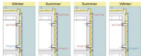
Mode of operation of the photovoltaic panels to supplement ventilation
