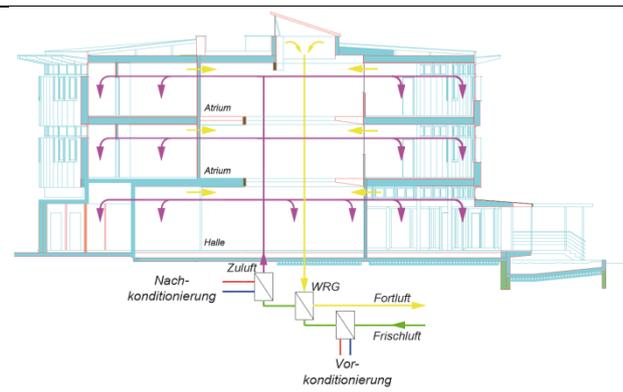
**Schematic diagram of the balanced mechanical air distribution system**
