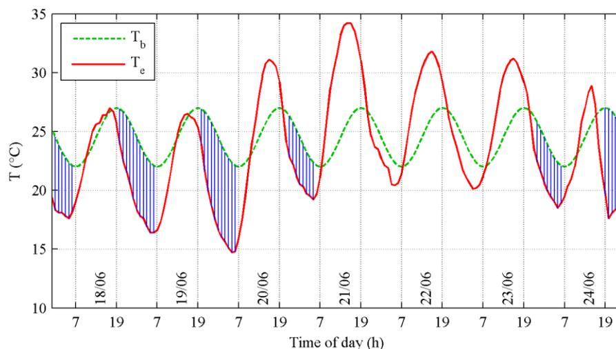
**Figure 2.4.** Building temperature,  $T_b$  and external air temperature,  $T_e$  during one week in summer 2003 for Zurich SMA (ANETZ data). Shaded areas illustrate graphically the climatic cooling potential, CCP. [13]
