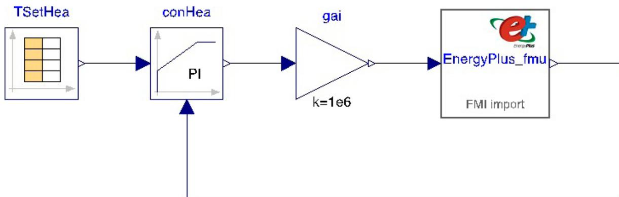
Figure 3: Modelica system model that connect a feedback controller with an EnergyPlus whole building model, which has been exported as an FMU.
