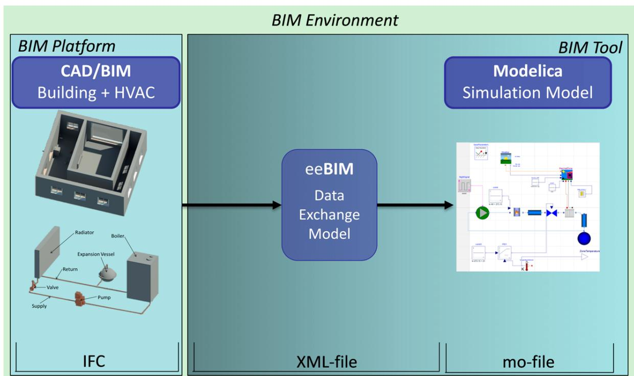
Figure 4: Overview of BIM transformation process from ifcXML to Modelica.
