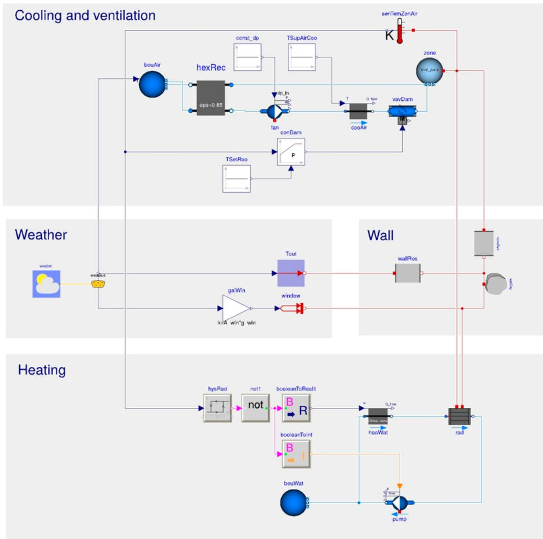
Figure 2: Modelica system model that shows a simple cooling and ventilation system (top), weather-driven heat gains, losses and storage (middle) and an idealized heating system (bottom).
