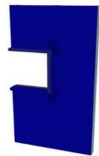
The wood buck needs to be sealed at the corners and connected with self adhesive membrane to the air/water control membrane
