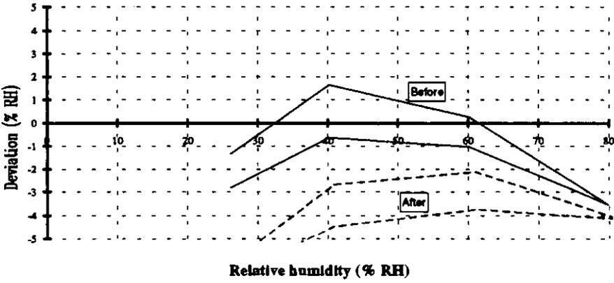
Characteristic curve for S15-RH before and after field testing in an office building
