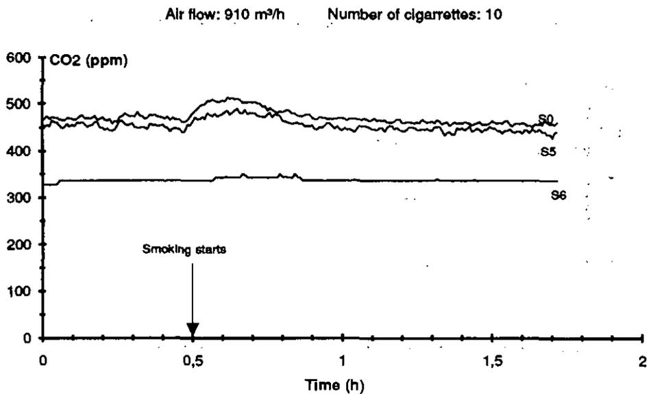
*Figure 5.20. Output of VOC- and CO<sub>2</sub>-sensors during tests with tobacco smoke. The ventilation flowrate was 910 m<sup>3</sup>/h and 10 cigarettes were smoked simultaneously on one occasion.*
