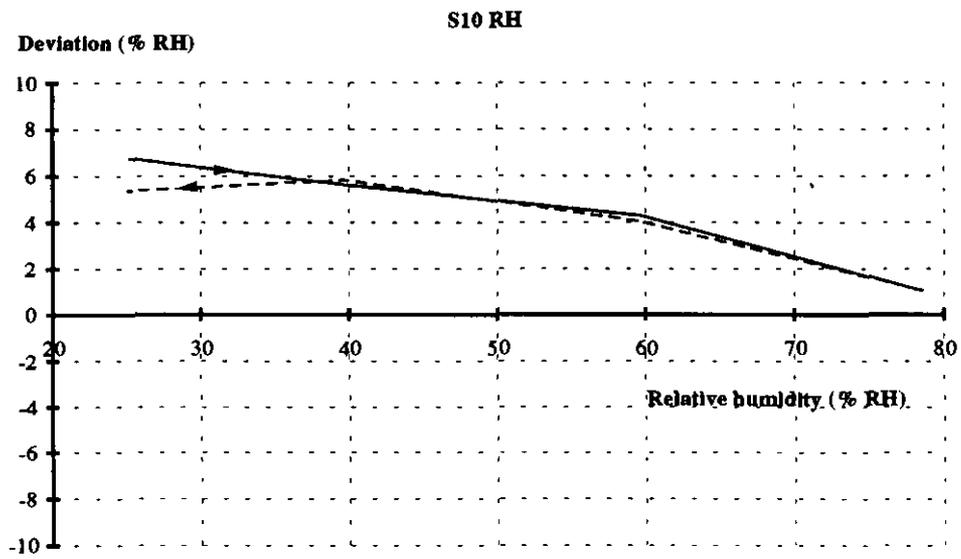
Figure 5.9. Characteristic curve for sensor S10.
