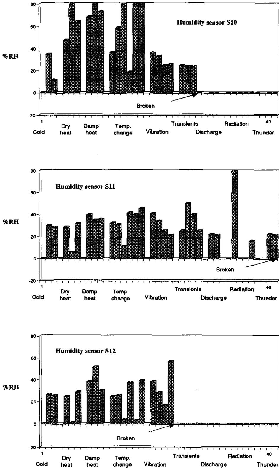
Figure 5.30. The output signals of humidity sensors S10, S11 and S12 during the environmental tests.
