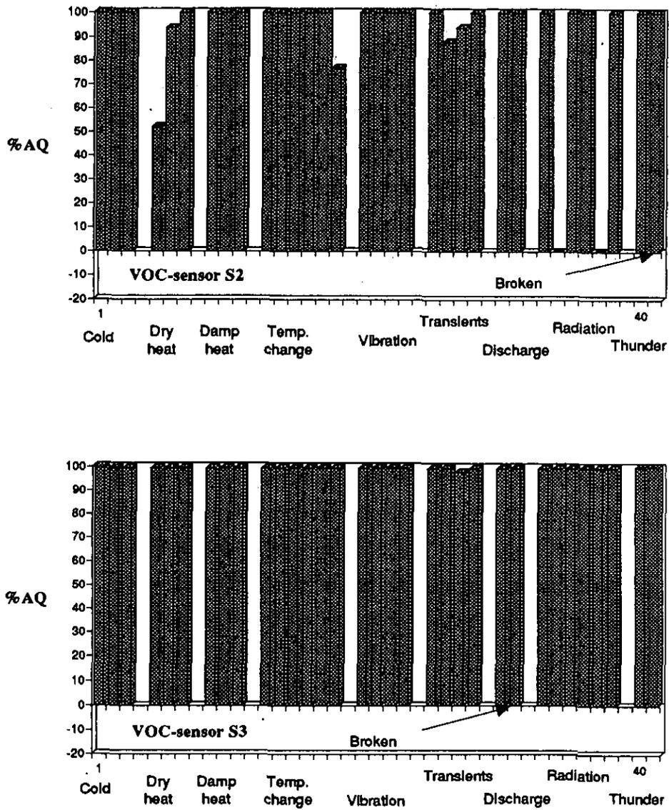
Figure 5.26. The output signals of VOC-sensors S2 and S3 during the environmental tests.
