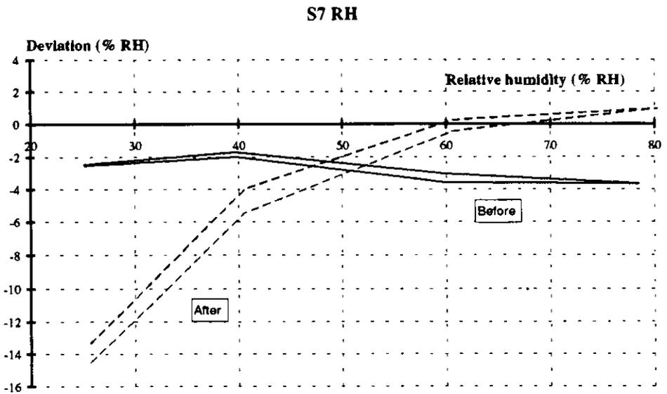
Figure 5.32. The characteristic curve of sensor S7 before and after the environmental test program (continuous and dashed curves respectively).
