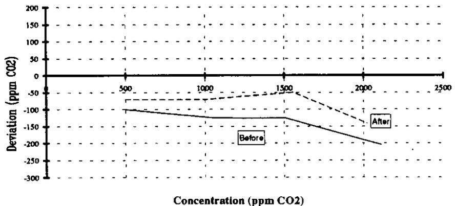
Figure 5.34. The characteristic curve of one sensor of the type S6 before and after 11 months of installation. Only one was delivered and this was installed in a conference room.
