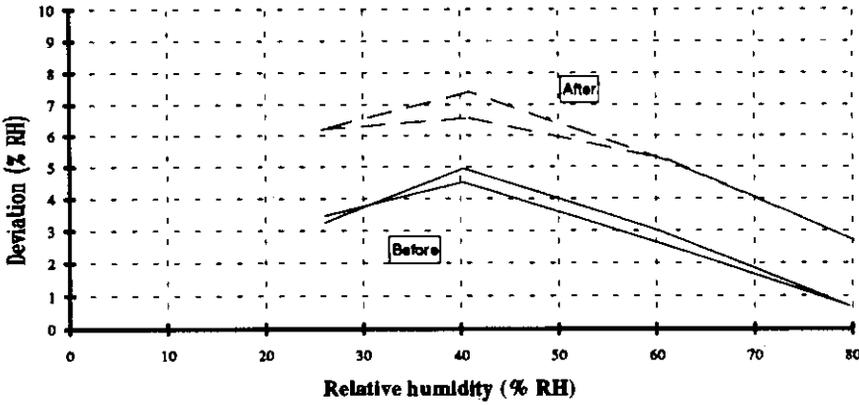
Characteristic curve for S11-RH before and after field testing in a calibration room
