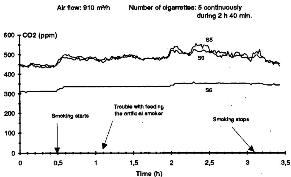
*Figure 5.22. Output of VOC- and CO<sub>2</sub>-sensors during tests with tobacco smoke. The ventilation flowrate was 910 m<sup>3</sup>/h and 5 cigarettes were smoked continuously during 2 h 40 minutes.*
