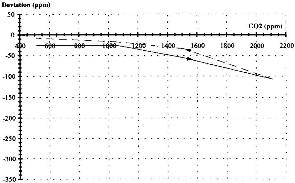
Figure 5.5. Characteristic curve for sensor S6.
