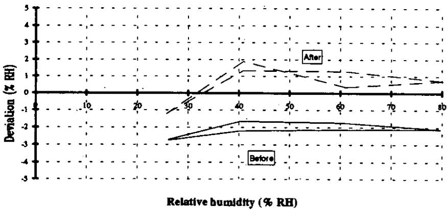
Characteristic curve for S12-RH before and after field testing in a calibration room
