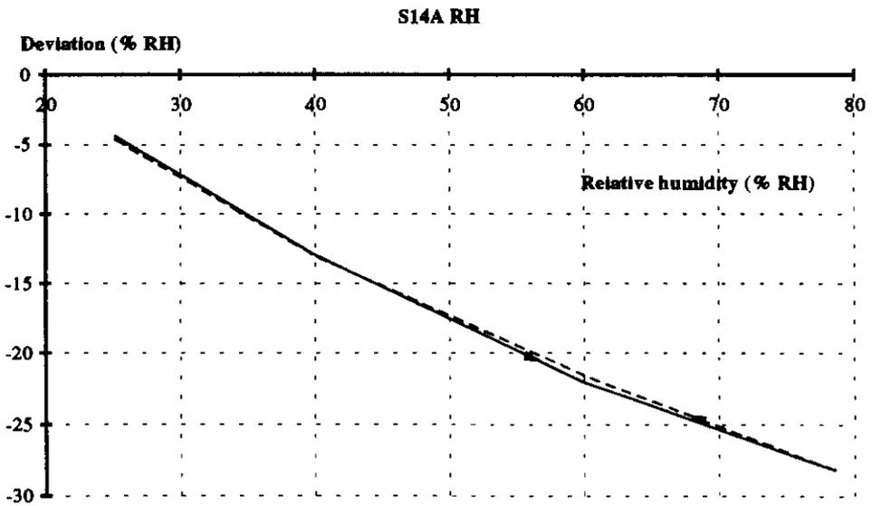
Figure 5.13. Characteristic curve for the RH-sensor in sensor S14, i.e. S14A.
