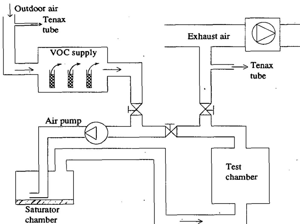
Figure A:2.7. The test set up used for VOC-sensors.
