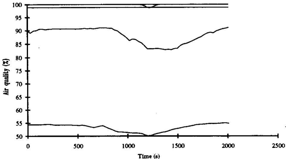
Figure 6.1. Output signals in terms of "percentage air quality" for sensors S1 - S4 and S14B as a function of time. The VOC-level was aimed at  $3.5 \text{ mg/m}^3$  but the background level changes after 800 s.
