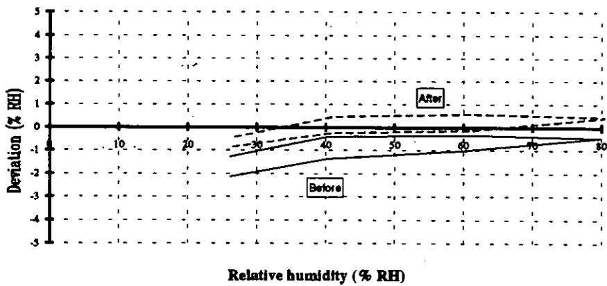
Characteristic curve for S12-RH before and after field testing in an office building
