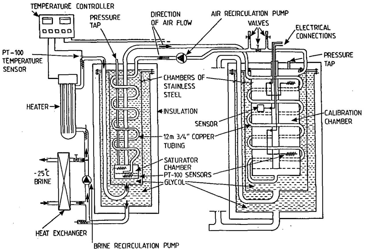
Figure A2.1. A schematic diagram of the two temperature type humidity calibrator.
