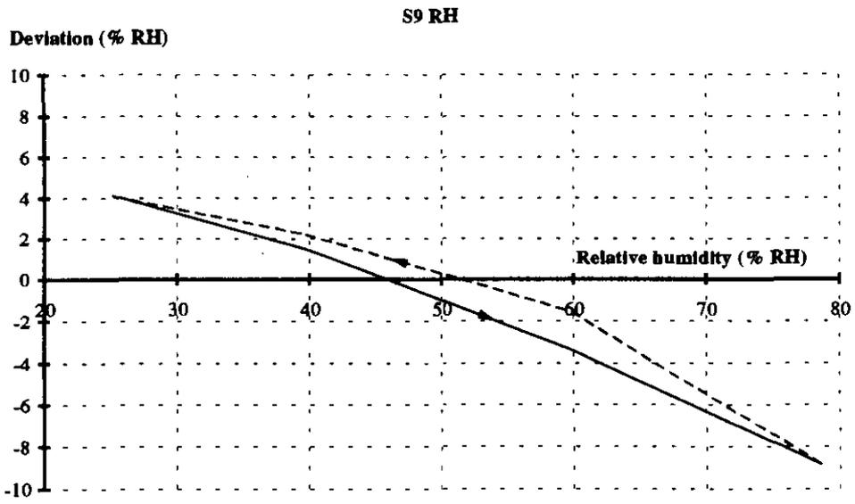
Figure 5.8. Characteristic curve for sensor S9.
