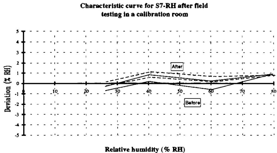
*Figure 5.36. Characteristic curves of sensors of the type S7 before and after 11 months of installation. One was installed in a conference room, one in an office and one in a calibration room respectively.*
