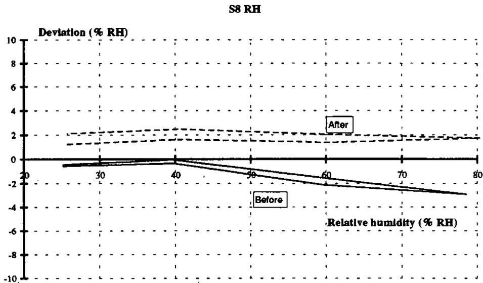
*Figure 5.33. The characteristic curve of sensor S8 before and after the environmental test program (continuous and dashed curves respectively).*
