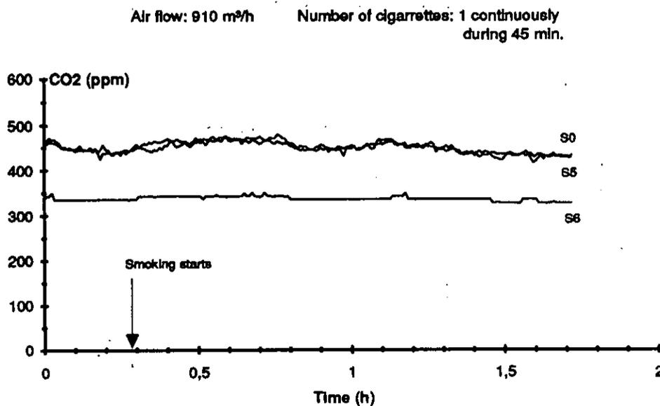
*Figure 5.21. Output of VOC- and CO<sub>2</sub>-sensors during tests with tobacco smoke. The ventilation flowrate was 910 m<sup>3</sup>/h and 1 cigarette was smoked continuously during 45 minutes.*
