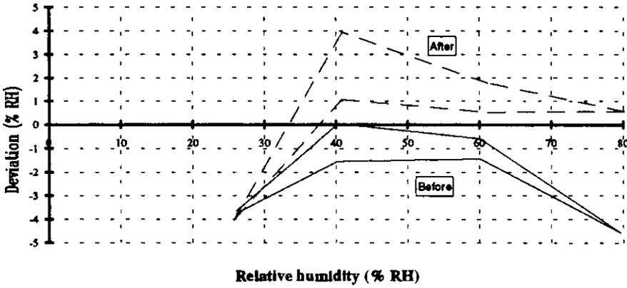
Characteristic curve for S15-RH before and after field testing in a calibration room
