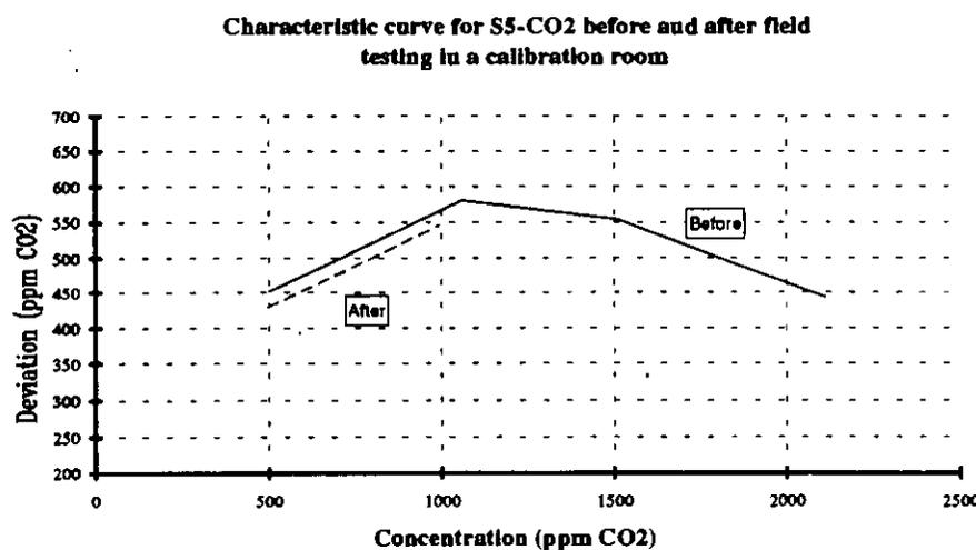
Figure 5.35. Characteristic curves of sensors of the type S5 before and after 11 months of installation. One was installed in a conference room, one in an office and one in a calibration room respectively. The dashed curve disappears outside the format of the bottom diagram.
