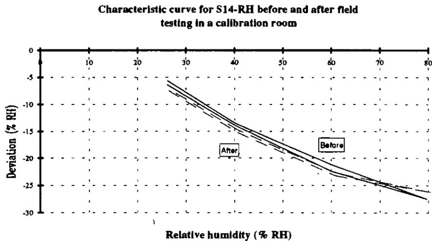
*Figure 5.43. Characteristic curves of sensors of the type S14A before and after 11 months of installation. One was installed in a conference room, one in an office and one in a calibration room respectively.*
