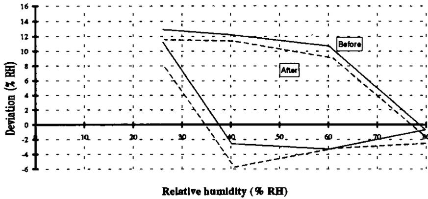
Characteristic curve for S10-RH before and after field testing in an office building
