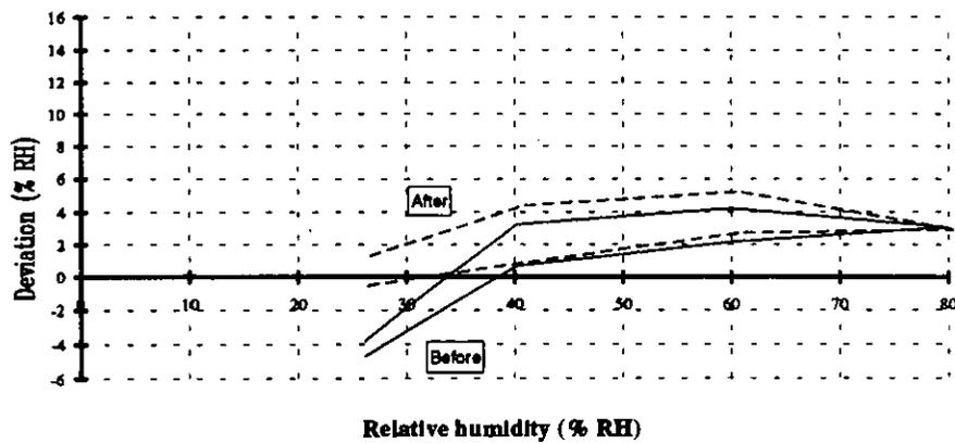
Figure 5.39. Characteristic curves of sensors of the type S10 before and after 11 months of installation. One was installed in a conference room, one in an office and one in a calibration room respectively.
