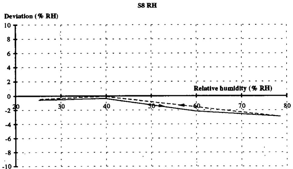
Figure 5.7. Characteristic curve for sensor S8.
