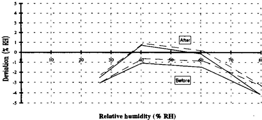
Figure 5.44. Characteristic curves of sensors of the type S15 before and after 11 months of installation. One was installed in a conference room, one in an office and one in a calibration room respectively.
