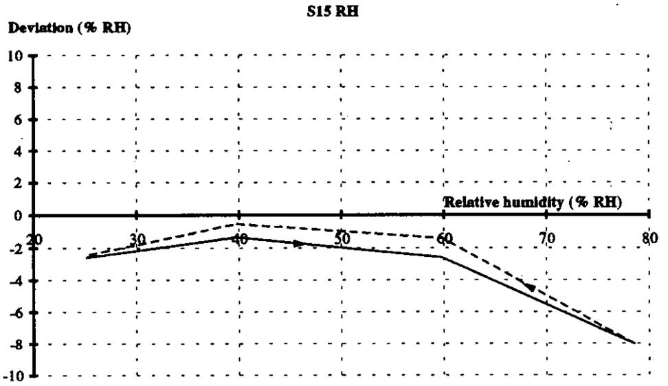
*Figure 5.14. Characteristic curve for sensor S15.*
