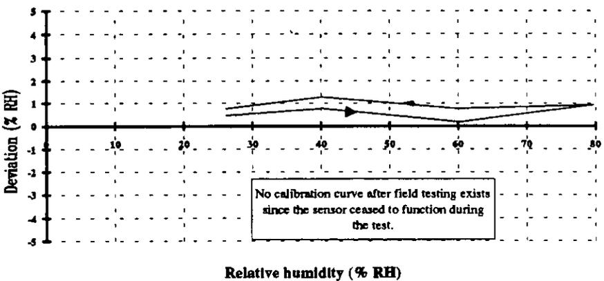
Figure 5.37. Characteristic curves of sensors of the type S8 before and after 11 months of installation. One was installed in a conference room, one in an office and one in a calibration room respectively.
