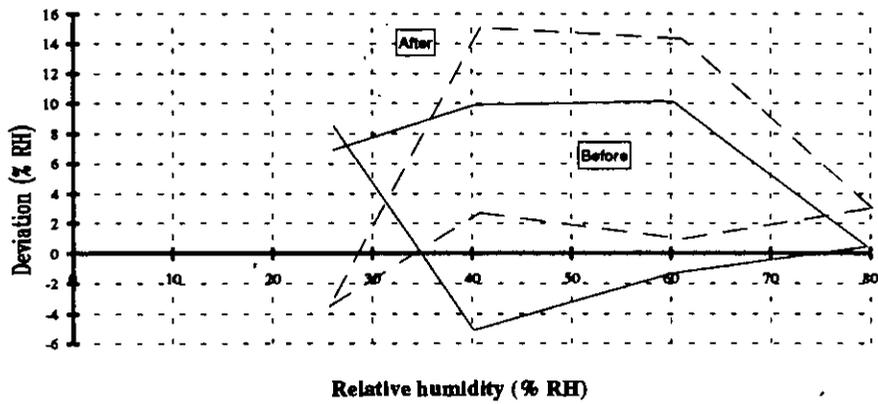
Characteristic curve for S10-RH before and after field testing in a calibration room
