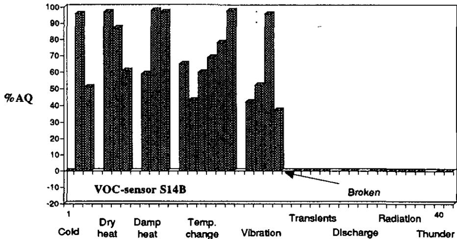
Figure 5.27. The output signals of VOC-sensors S4 and S14B during the environmental tests.
