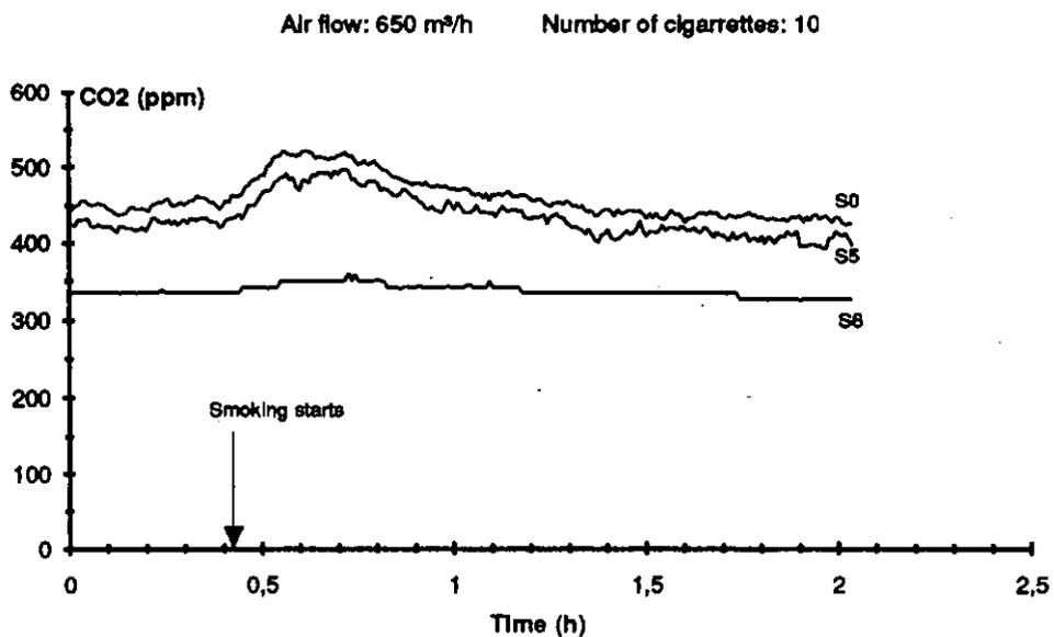
Figure 5.18. Output of VOC- and CO<sub>2</sub>-sensors during tests with tobacco smoke. The ventilation flowrate was 650 m<sup>3</sup>/h and 10 cigarettes were smoked simultaneously on one occasion.
