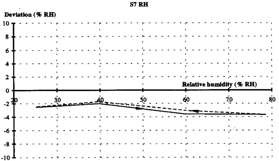
Figure 5.6. Characteristic curve for sensor S7.
