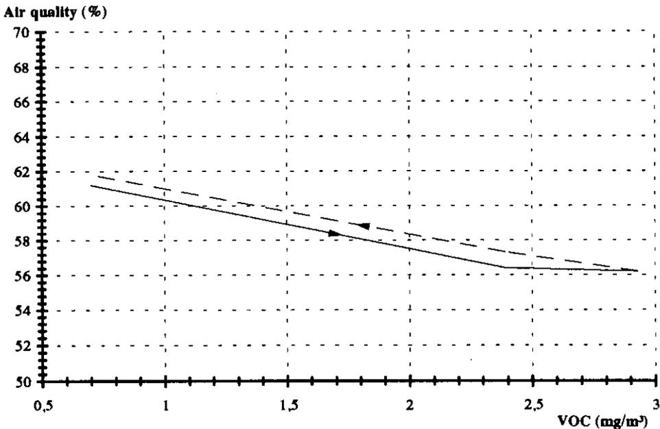
Figure 5.1. Characteristic curve for sensor S1.
