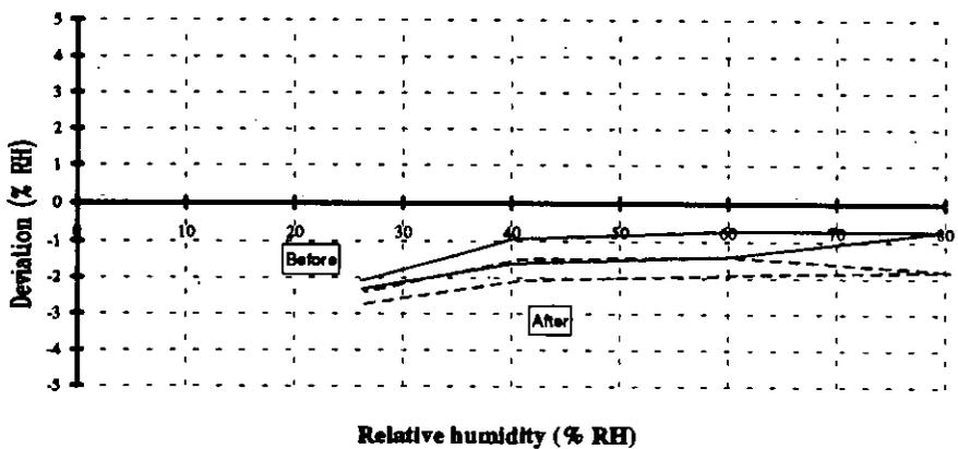
Figure 5.41. Characteristic curves of sensors of the type S12 before and after 11 months of installation. One was installed in a conference room, one in an office and one in a calibration room respectively.
