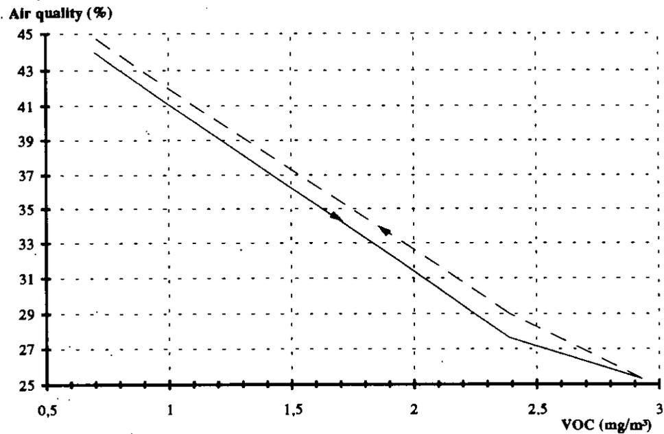
Figure 5.3. Characteristic curve for the VOC-sensor in sensor S14B.
