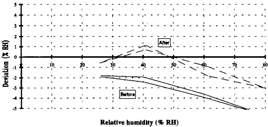
Characteristic curve for S13-RH before and after field testing in a calibration room
