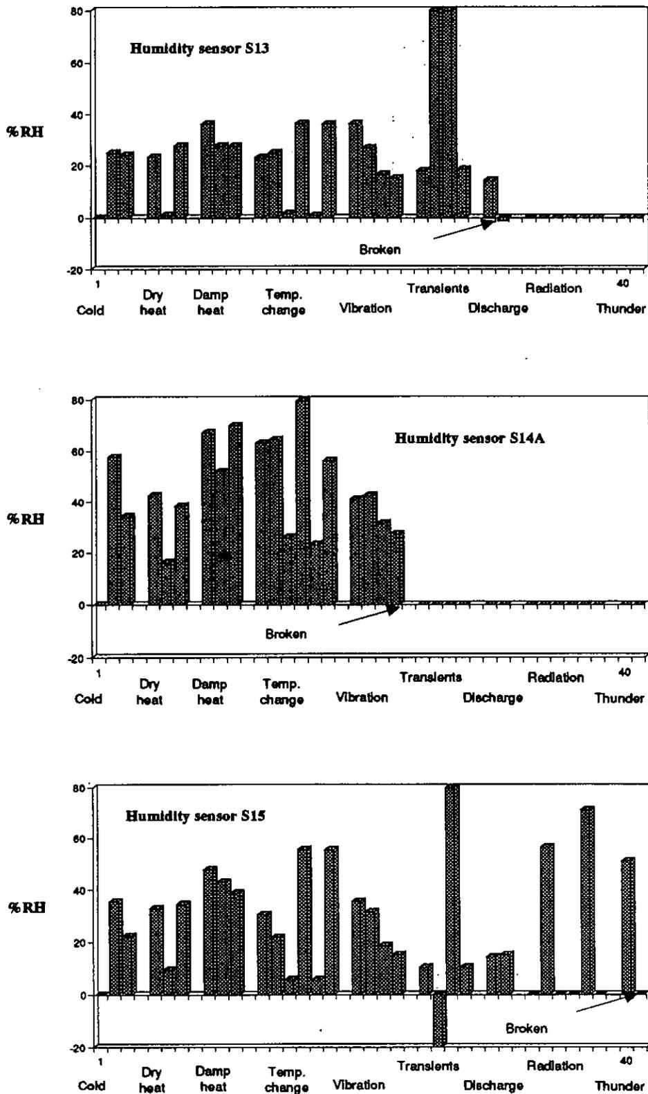
Figure 5.31. The output signals of humidity sensors S13, S14A and S15 during the environmental tests.
