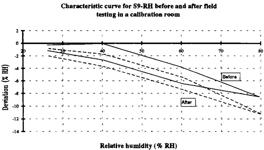
*Figure 5.38. Characteristic curves of sensors of the type S9 before and after 11 months of installation. One was installed in a conference room, one in an office and one in a calibration room respectively.*
