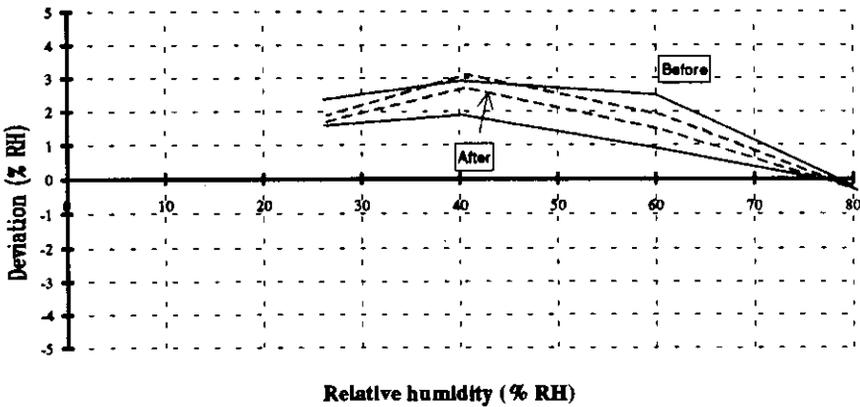
Figure 5.40. Characteristic curves of sensors of the type S11 before and after 11 months of installation. One was installed in a conference room, one in an office and one in a calibration room respectively.
