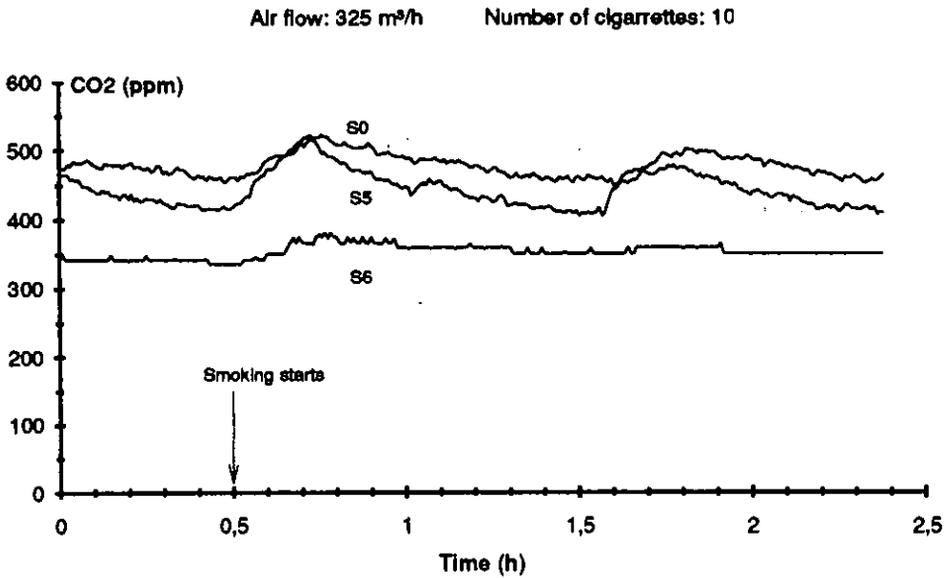
Figure 5.16. Output of VOC- and CO<sub>2</sub>-sensors during tests with tobacco smoke. The ventilation flowrate was 325 m<sup>3</sup>/h and 10 cigarettes were smoked simultaneously on one occasion.
