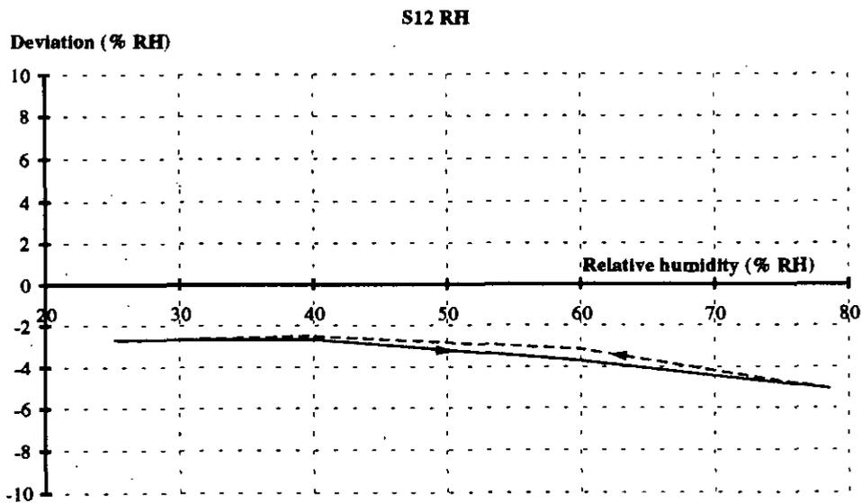
Figure 5.11. Characteristic curve for sensor S12.
