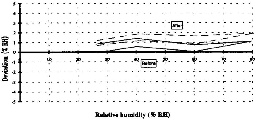
Characteristic curve for S8-RH before and after field testing in an office building
