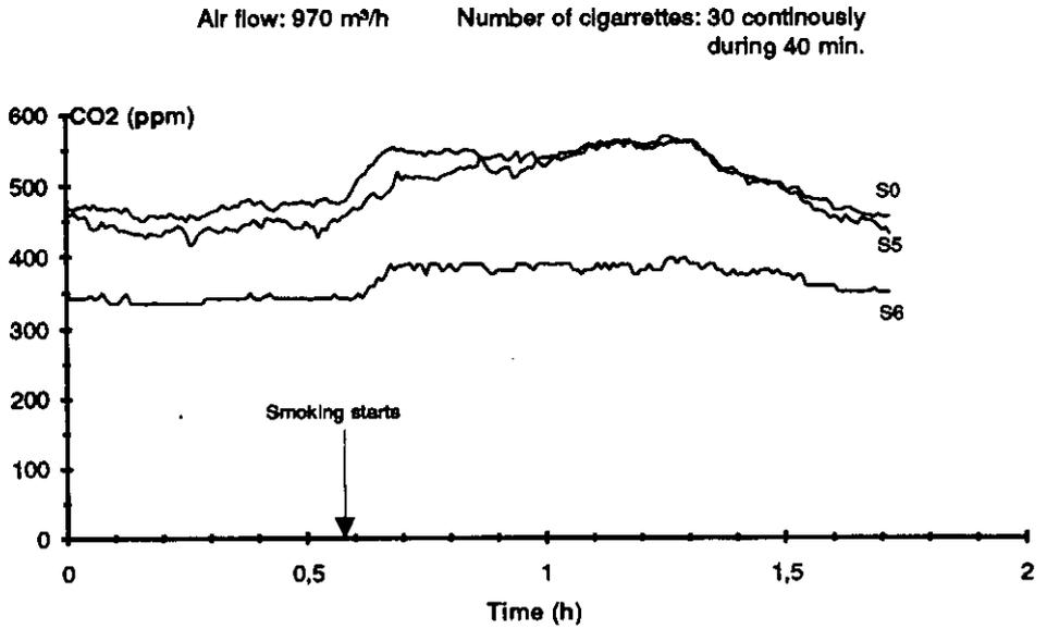
Figure 5.24. Output of VOC- and CO<sub>2</sub>-sensors during tests with tobacco smoke. The ventilation flowrate was 970 m<sup>3</sup>/h and 30 cigarettes were smoked continuously during 40 minutes.
