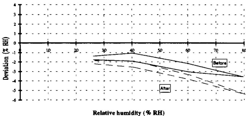
Figure 5.42. Characteristic curves of sensors of the type S13 before and after 11 months of installation. One was installed in a conference room, one in an office and one in a calibration room respectively.
