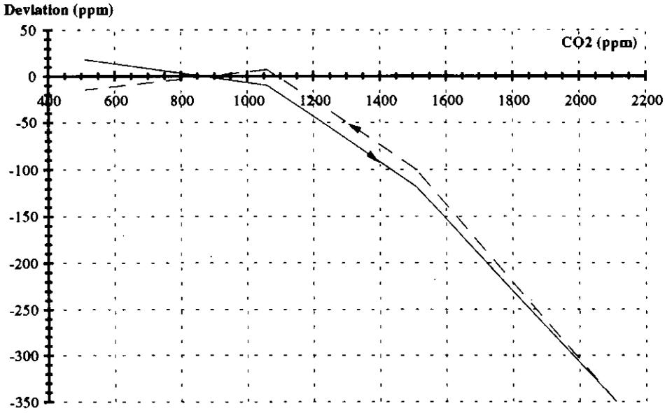
Figure 5.4. Characteristic curve for sensor S5.
