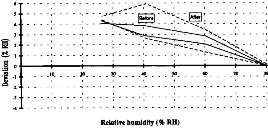
Characteristic curve for S11-RH before and after field testing in an office building
