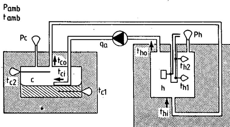
Figure A2.6. Measuring positions in the humidity calibrator.
