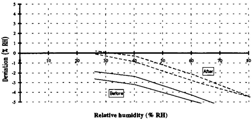
Characteristic curve for S13-RH before and after field testing in an office building
