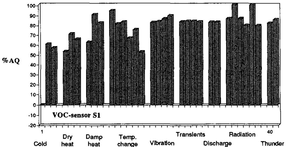
Figure 5.25. The output signal of VOC-sensor S1 during the environmental tests.
