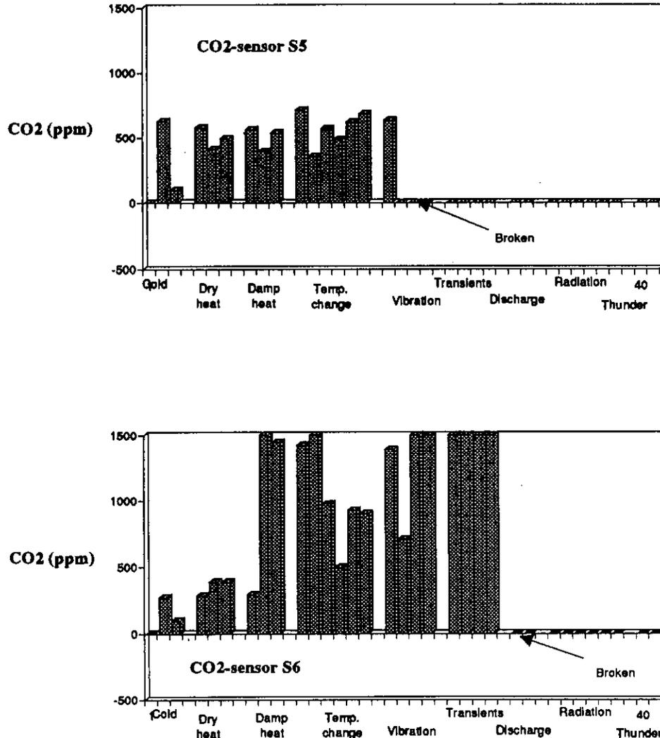
Figure 5.28. The output signals of carbon dioxide sensors S5 and S6 during the environmental tests.
