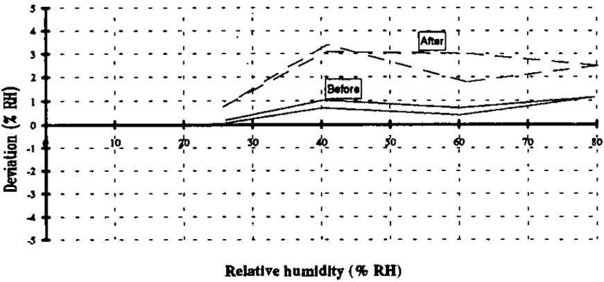
Characteristic curve for S8-RH before field testing in a calibration room
