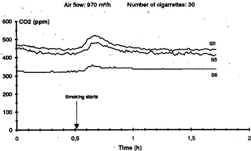
Figure 5.23. Output of VOC- and CO<sub>2</sub>-sensors during tests with tobacco smoke. The ventilation flowrate was 970 m<sup>3</sup>/h and 30 cigarettes were smoked simultaneously on one occasion.
