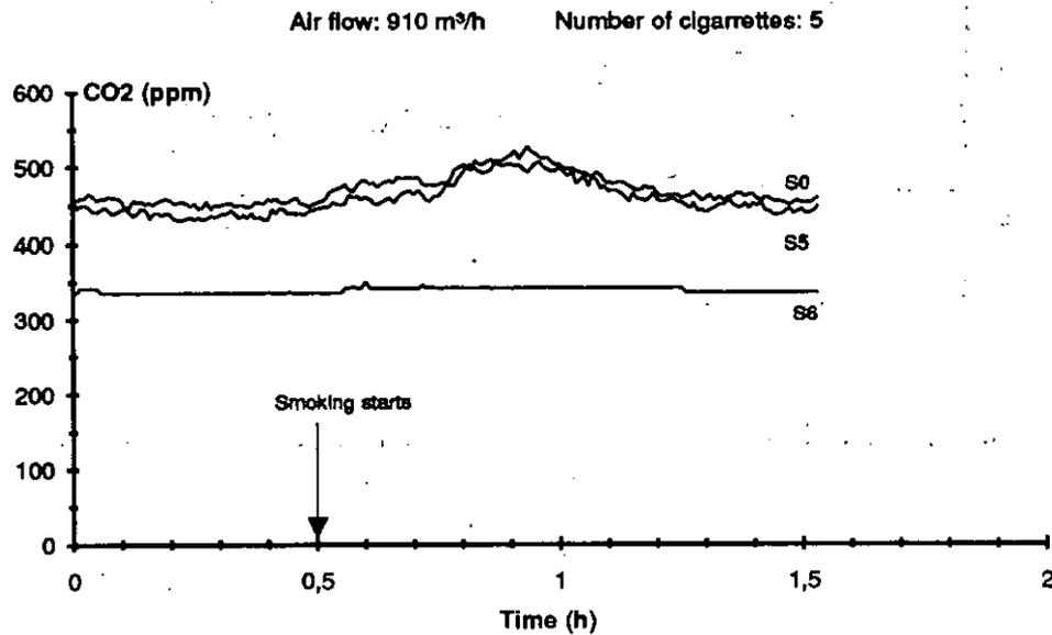
Figure 5.19. Output of VOC- and CO<sub>2</sub>-sensors during tests with tobacco smoke. The ventilation flowrate was 910 m<sup>3</sup>/h and 5 cigarettes were smoked simultaneously on one occasion.
