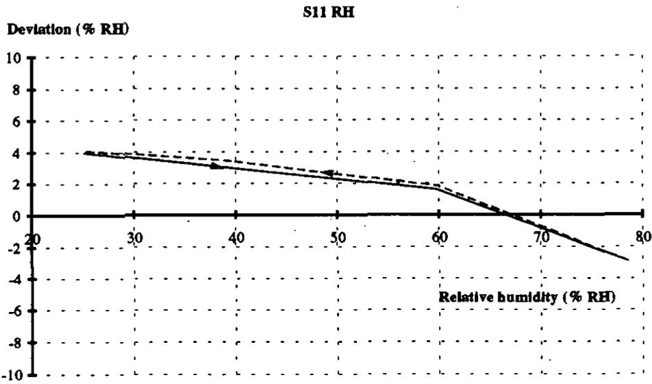
Figure 5.10. Characteristic curve for sensor S11.
