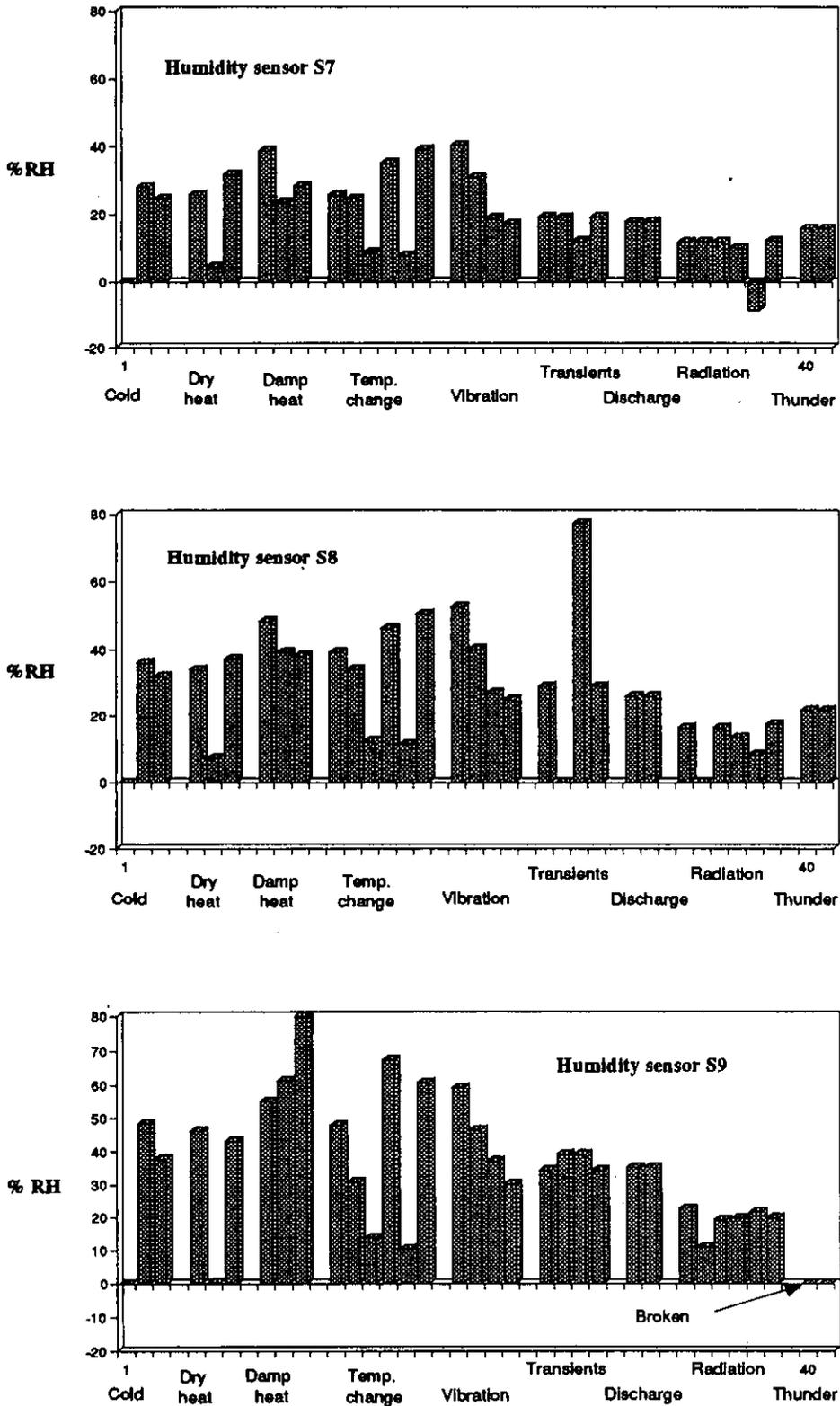
Figure 5.29. The output signals of humidity sensors S7, S8 and S9 during the environmental tests.
