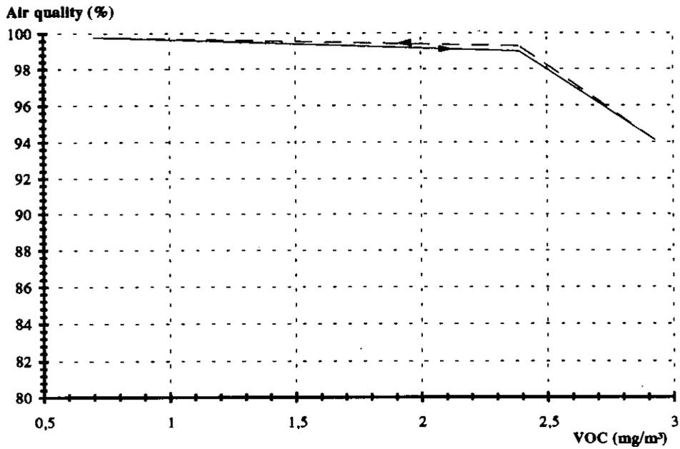
Figure 5.2. Characteristic curve for sensor S4 .
