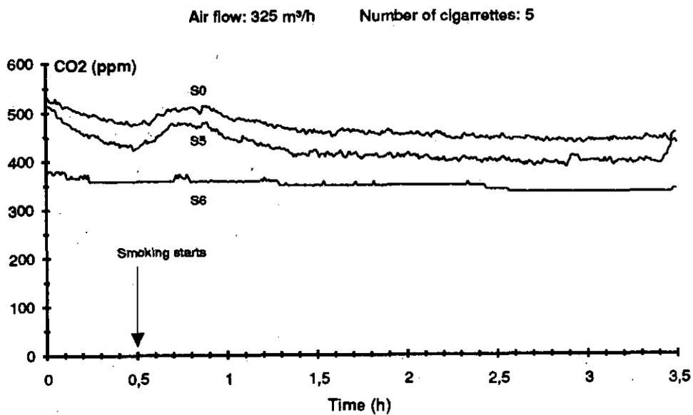
Figure 5.15. Output of VOC- and CO<sub>2</sub>-sensors during tests with tobacco smoke. The ventilation flowrate was 325 m<sup>3</sup>/h and 5 cigarettes were smoked simultaneously on one occasion.
