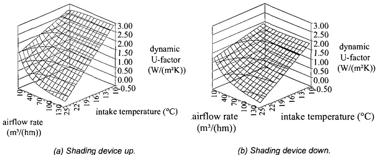
Figure 6.4 The dynamic U-value of the envelope shown in Figure 6.3 as a function of air flow rate and intake air temperature.
