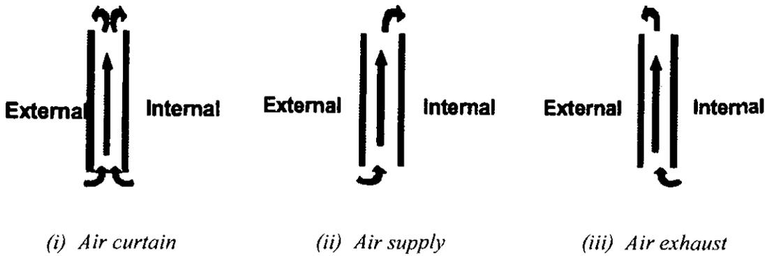
Figure 6.2 Possible air flow arrangements in an active envelope
