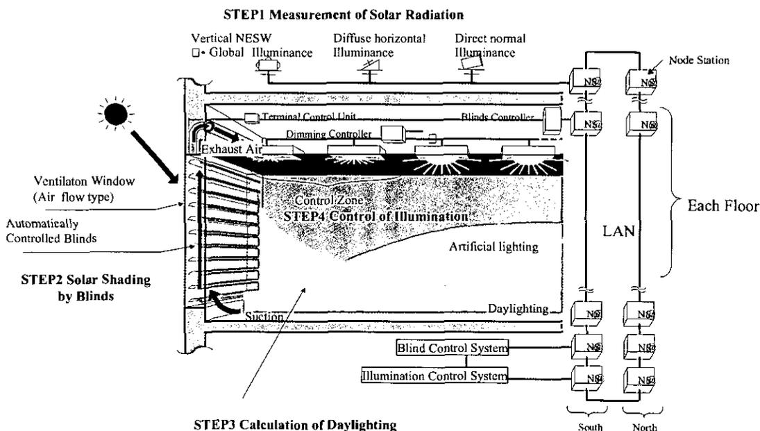
Figure 6.6 Schematic arrangement of the active window and illumination control system – TEPCO Research and Development Centre, Tokyo.
