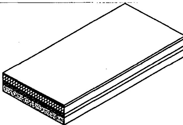
Figure 5.1 Flat roof insulation system using a concrete deck and rigid insulation boards, separated by a vapour barrier
