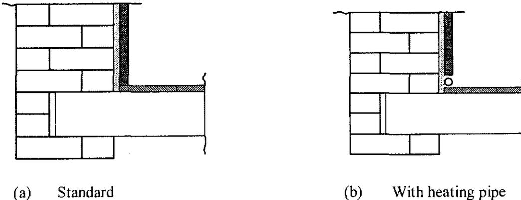
Figure 5.4 Junction between masonry wall with internal insulation and timber floor
