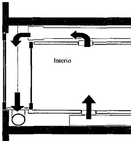
Figure 6.3 Schematic diagram of an 'active window' system
