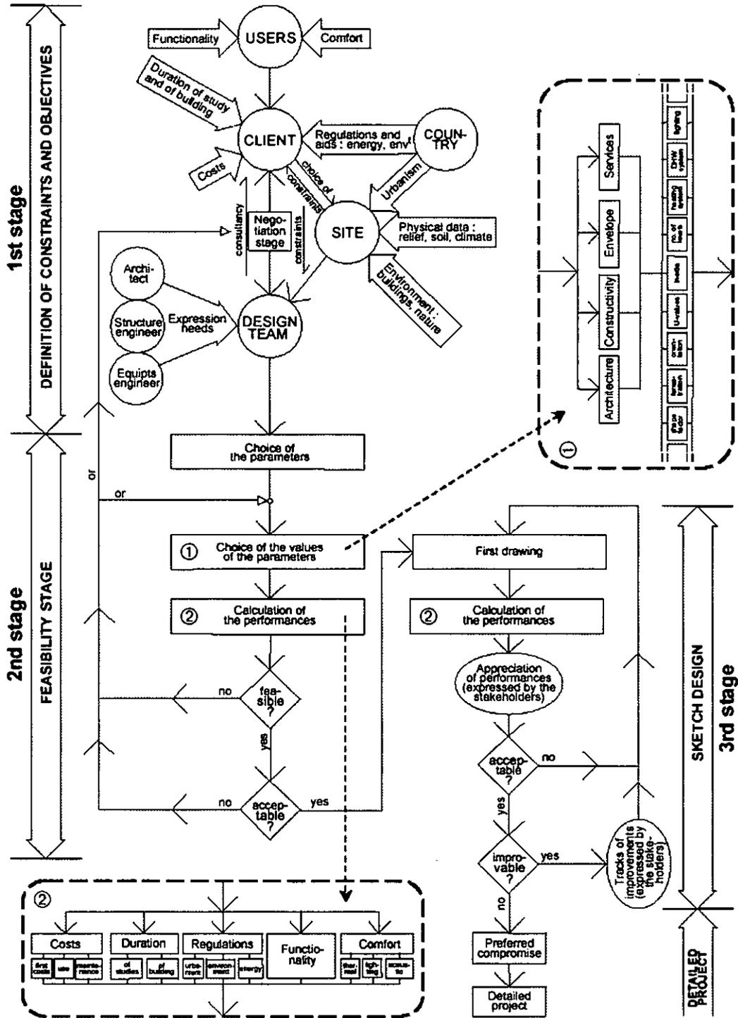
Figure 3.4 Interactions during the preliminary stages of the design process
