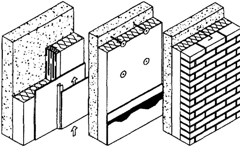
Figure 5.3 External insulation systems – Type A, Type K and Type L
