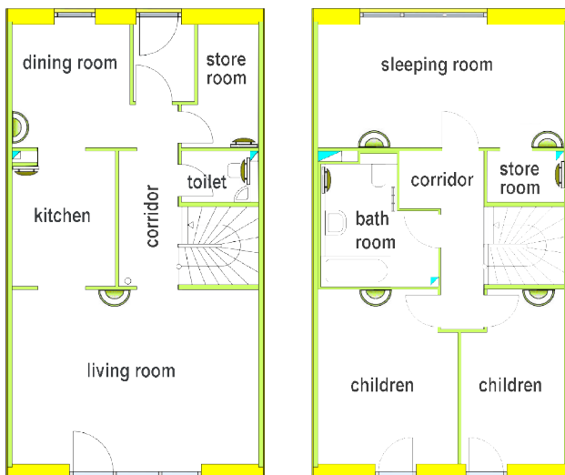
horizontal projection supply-air and exhaust-air valves are indicated
