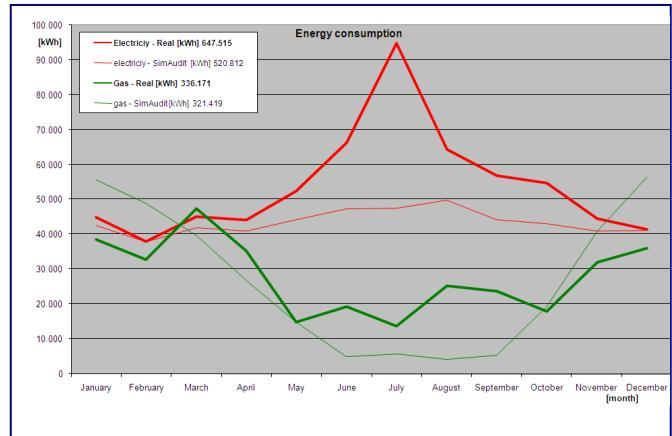
Comparison between the simulated energy consumptions (thin lines) and the measured ones (thick lines). Gas is red, electricity is green.
