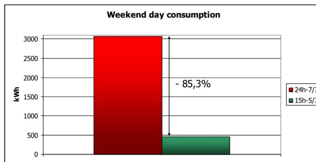
Mean difference on electric consumption between different VRF system schedules
