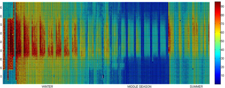
Carpet plots of building global electric consumption. The value are in kWh and refers to sampling time of 15 minutes
