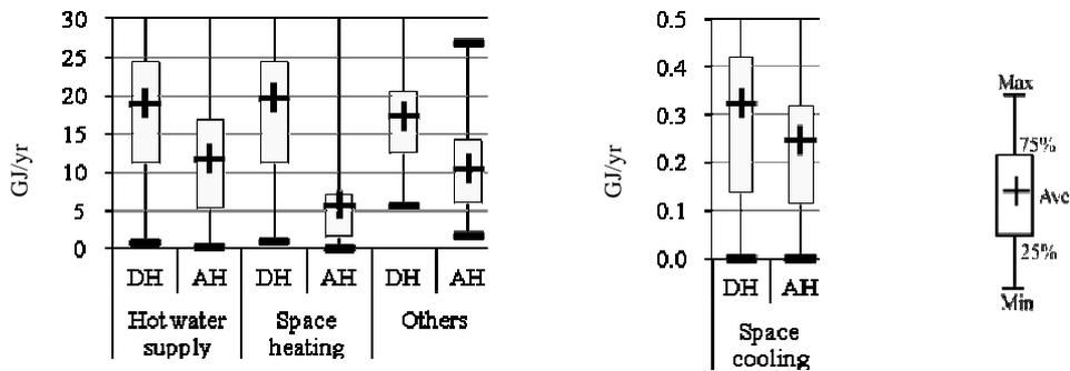
Figure 2-85: Energy consumption for each end use
