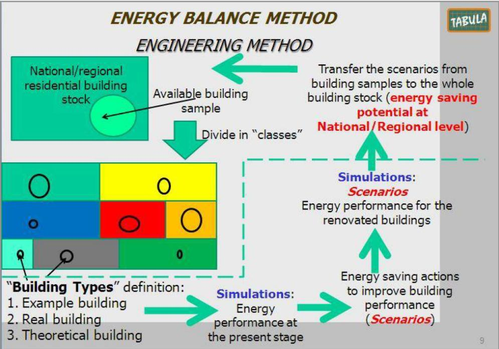
Figure 2-139: Procedure for Energy Balance Method used in the TABULA project to predict the potential impact of energy efficiency measures on national housing sector.
