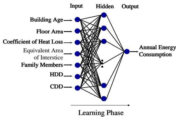
Figure 2-113: Input and output layers in neural network
