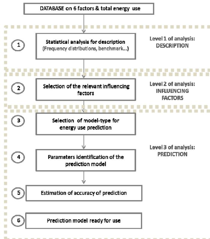
Figure 2-1: “Stages of development a model for prediction the total energy use in buildings”
