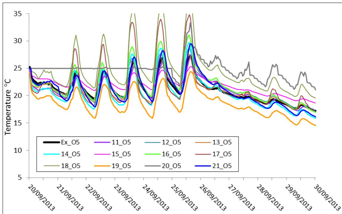
Figure 22: Experiment 1 Blind validation. Living room temperature: Free-float period: models 11-21 + experimental data: House O5
