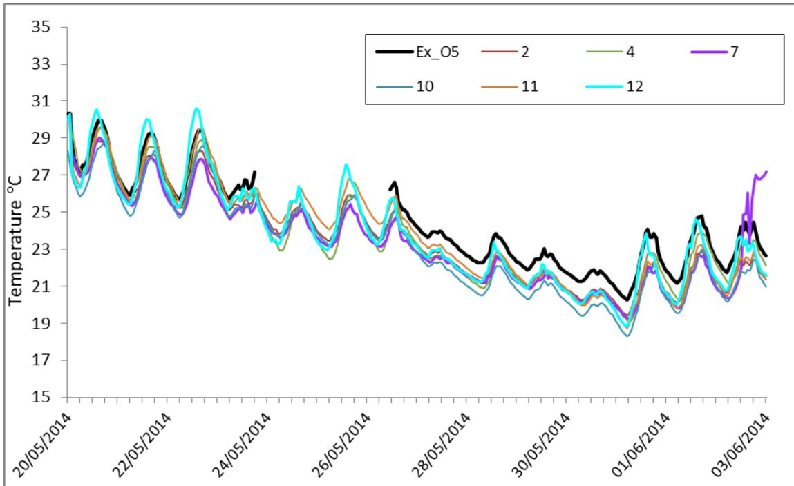
Figure 30: Experiment 2: Living room temperature: Free-float period: 6 models + experimental data: House O5
