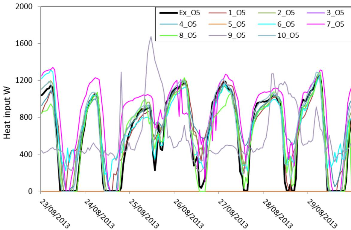
Figure 17: Experiment 1 Blind validation. Living room heat input: constant temperature phase (30°C): models 1-10 + experimental data: House O5
