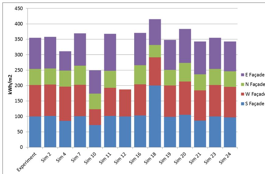
Figure 34: Experiment 2: cumulative solar irradiation
