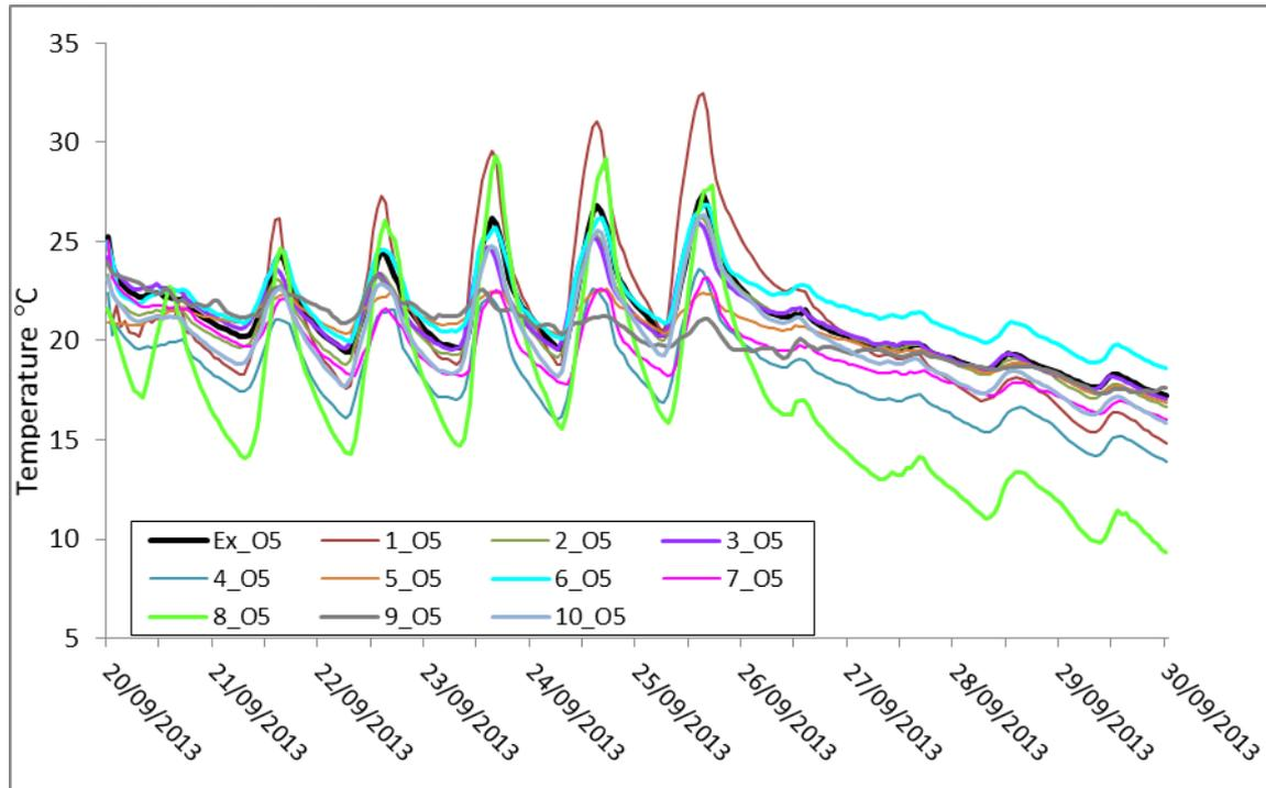
Figure 21: Experiment 1 Blind validation. Living room temp: Free-float period: models 1-10 + experimental data: House O5
