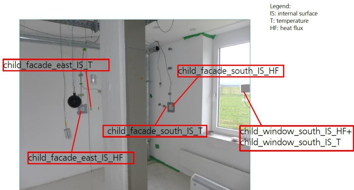
Figure 10: Heat flux and surface temperature sensors in the south bedroom (also called children's room)
