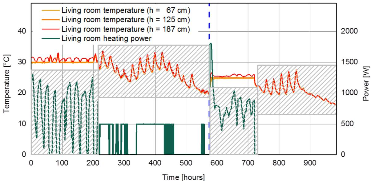
Figure 16: Profiles of the heating power and the air temperature at all three measurement heights of the living room of one of the houses. The grey shaded data are the validation targets that are not provided for the blind validation.
