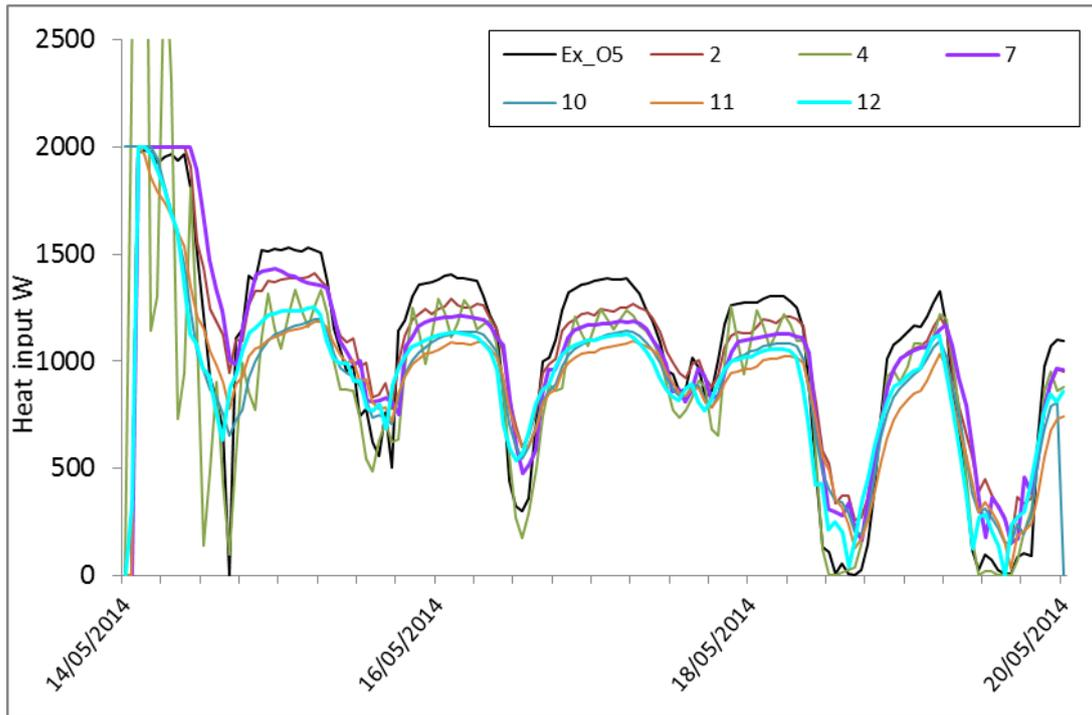
Figure 26: Experiment 2: Living room heat input: constant temperature phase (30°C): 6 models + experimental data: House O5
