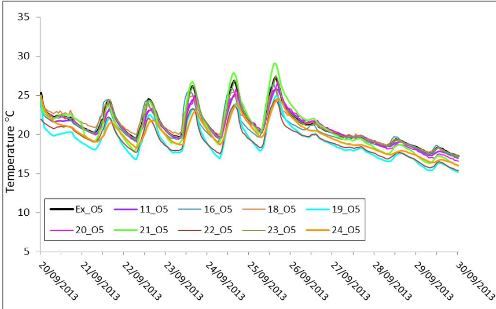
Figure 24: Experiment 1 Re-modelling. Living room temperature: Free-float period: another 9 models + experimental data: House O5
