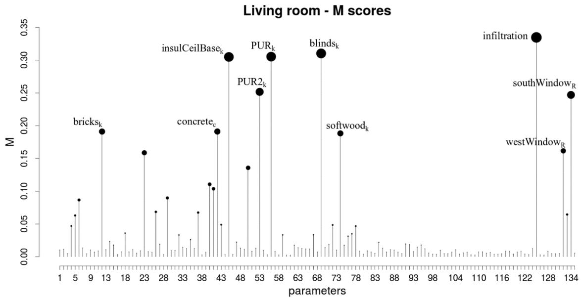
Figure 36:  $M_i$  scores for the living room constant temperature period.  $R$ ,  $k$  and  $c$  indicate thermal resistance, conductivity and specific heat
