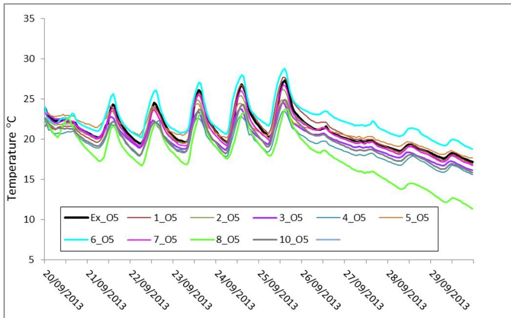
Figure 23: Experiment 1 Re-modelling. Living room temperature: Free-float period: 9 models + experimental data: House O5
