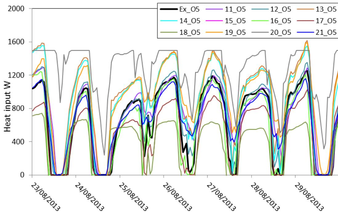
Figure 18: Experiment 1 Blind validation. Living room heat input: constant temperature phase (30°C): models 11-21 + experimental data: House O5
