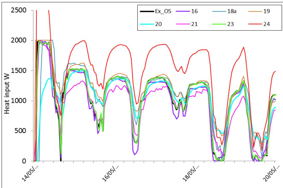
Figure 27: Experiment 2: Living room heat input: constant temperature phase (30°C): the other 7 models + experimental data: House O5
