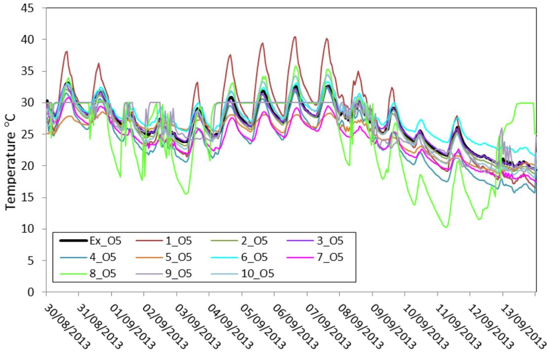
Figure 19: Experiment 1 Blind validation. Living room temperature: ROLBS sequence: models 1-10 + experimental data: House O5
