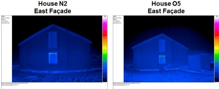
Figure 5 Thermal images of the East Facades of the two houses.
