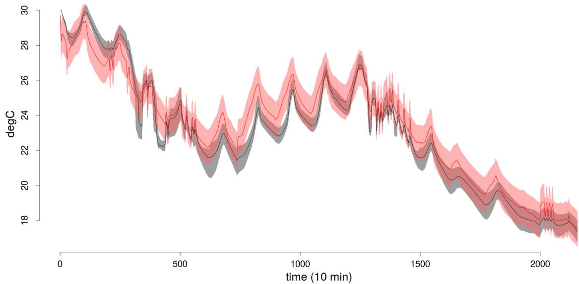
Figure 37: Mean values and 95% confidence bands for the living room measured (red) and predicted (black) internal temperature: ROLBS
