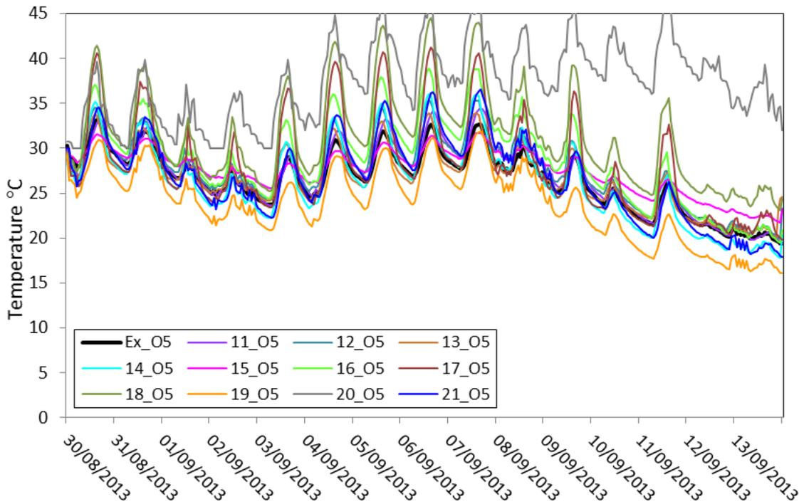
Figure 20: Experiment 1 Blind validation. Living room temperature: ROLBS sequence: models 11-21 + experimental data: House O5
