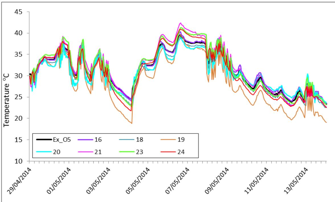
Figure 29: Experiment 2: Living room temperature: ROLBS sequence: the other 7 models + experimental data: House O5
