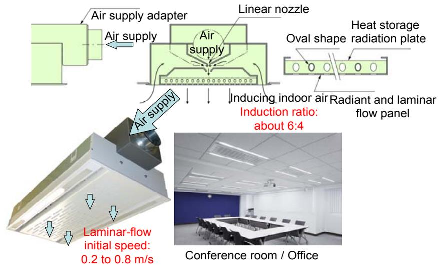
Fig. 4-28 Diagram of the all air supplied radiant and laminar flow unit (Induction air beam)
