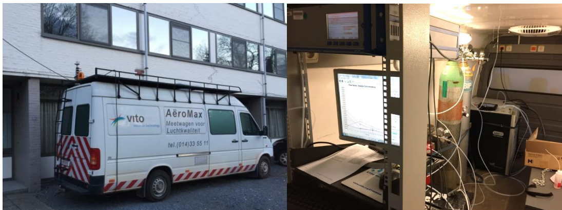
Figure 17 - VITO van containing the Sift MS and FID monitor.
