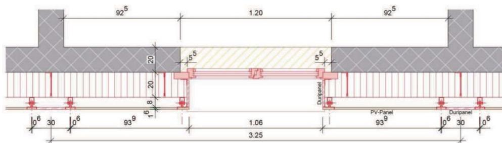
Figure 140: Cross section facade north, ©. Source: Baubüro in situ
