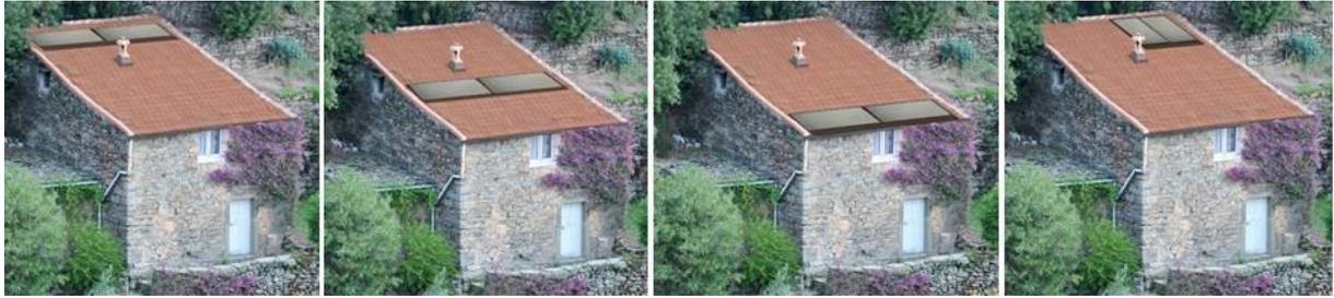
Figure 130: Schiara, study of the different impact of two thermal solar panels on a roof changing their position and alignment
