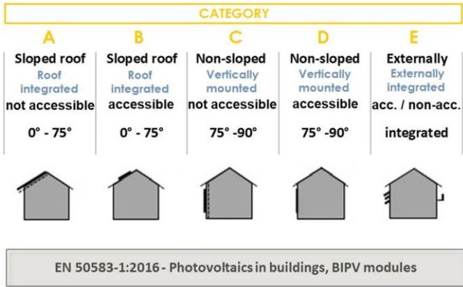
Figure 1: Mounting categories A – E (EN 50583-1:2016 - Photovoltaics in buildings - Part 1: BIPV modules)
