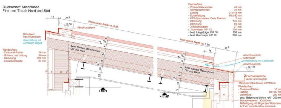
Figure 137: Cross section roof detail, © baubüro in situ
