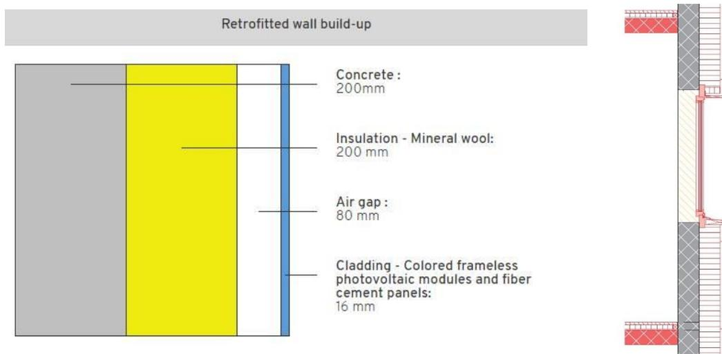
Figure 136: Cross section façade north. Source: © Baubüro in situ
