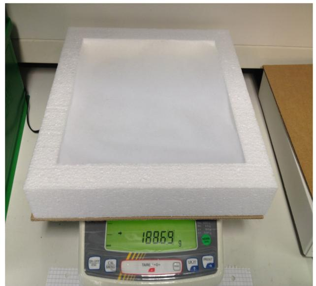
A specimen holder for loose-filled granulate, constructed from an expanded polystyrene frame, provided as an accessory from the manufacturer of thermal conductivity testing apparatus. Source: German Aerospace Center (DLR), 2017
