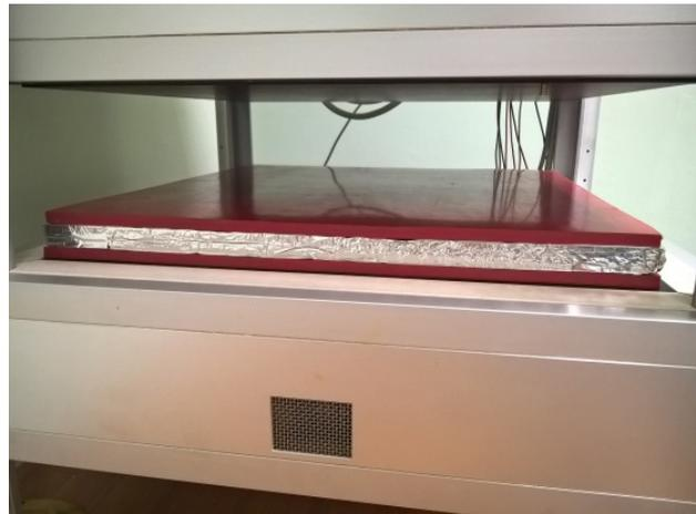
Extra layers of 10 mm thick rubber for measurement of vacuum insulation panels.
