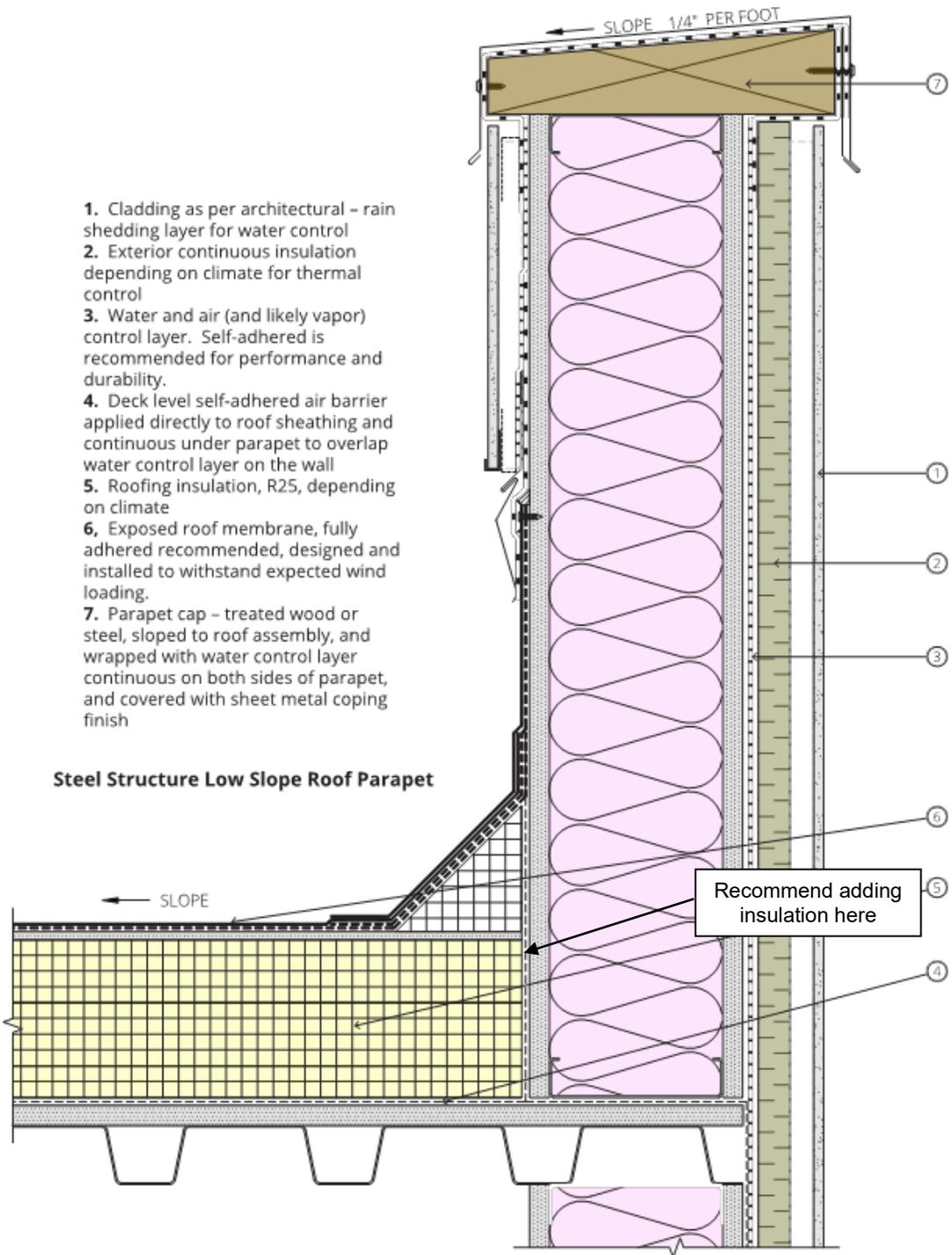
1. Cladding as per architectural – rain shedding layer for water control
