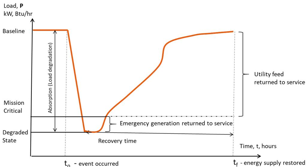
**Figure 3-5. Stepped recovery of power system assets.**
