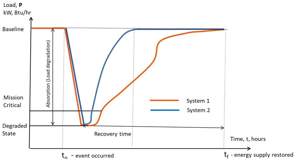
**Figure 3-4. Two systems with different recovery times.**
