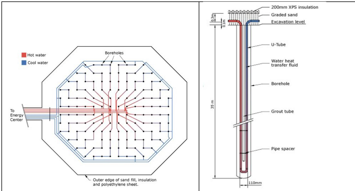
**Borehole Thermal Energy Storage (BTES) installed at Drake Landing Solar Community. 144 – 150 mm (6 in.) dia x 35 m (115 ft) deep boreholes spaced 2.25 m (7 ft) of center used for storing heat collected in summer for use later in winter (Drake Landing Solar Community (dlsc.ca).**
