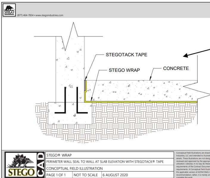
**Recommend installing vapor barrier to foundation wall.**
