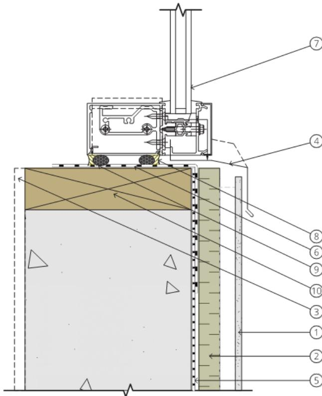
1. Cladding as per architectural – rain shedding layer for water control
