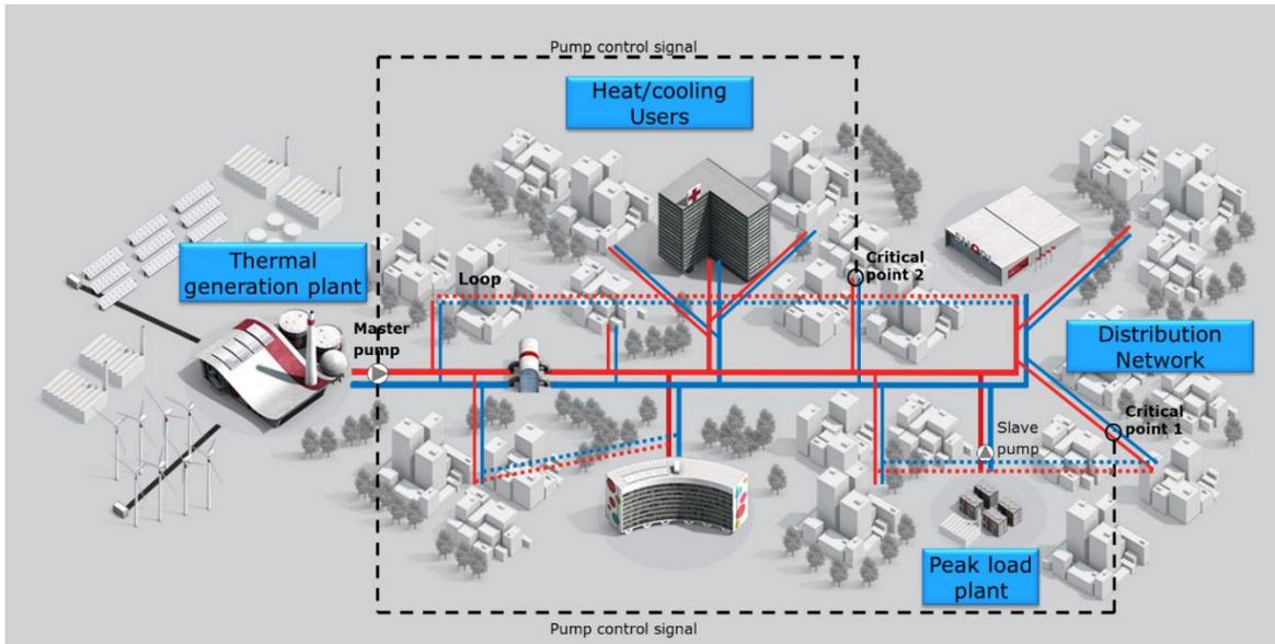
**Figure 6-14. Example of multi-thermal source and meshed network layout structure of a district energy system. The dotted lines represent the transformation from a branch to a meshed system type. The black lines represent pump control signals.**
