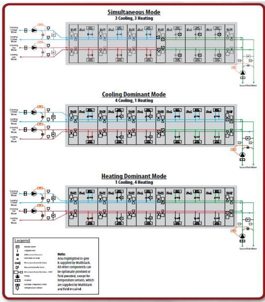
**Figure 5-14. MultiStack Virtual Movable End Cap System:** This system lends itself to ground-sink/ source operation if the real estate is available for the wells or other heat exchange fields. Large bodies of water would also be suited for use as sinks/sources if environmental regulations local to the proposed use will allow.
